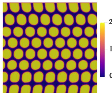
Fig. 9 Droplets moving in a channel. This was obtained using a free energy LBM and solving eqn (84). Colour depicts  $\sum_i \phi_i$  which is  $\approx 2$  for droplets (yellow) and  $\approx 0$  for the background fluid (black).
