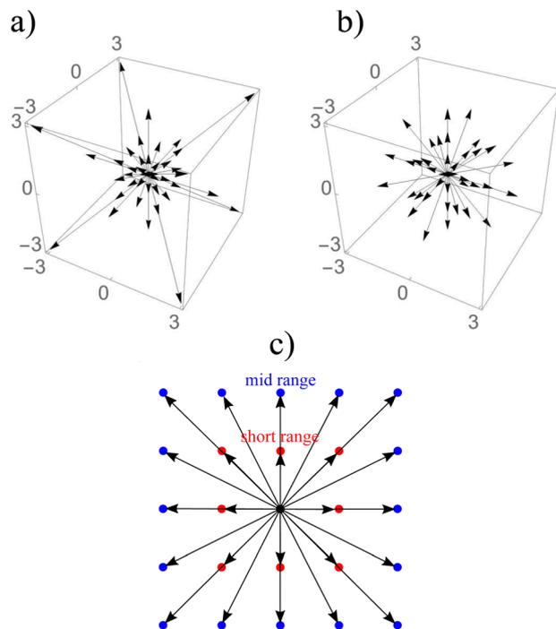
**Fig. 10** (a) The D3Q41 lattice and (b) the D3Q39 lattice. The D3Q41 is a zero-one-three lattice meaning that it is analogous to the Brillouin zones (also referred to as lattice-belts, or lattice-stencils) covered by  $\xi_x$ . The D3Q39 is a zero-one-two-three lattice. (c) The D2Q9 lattice for short-range nodes (red). The D2Q25 lattice for short and mid-range nodes (blue).
