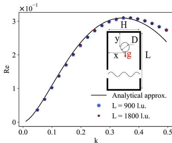
Fig. 12 Schematic of an initially circular particle of diameter  $D$  moving in a channel of length  $L$  and width  $H$  due to the force of gravity  $g$ . The particle is placed at  $x_0 = 0.5H$ . Terminal velocity  $V_t$  against dimensionless size  $k$ . The particle has a diameter of 12.5 l.u. and the fluid has a relaxation parameter  $\tau = 1$ . The analytical approximation corresponds to eqn (100).
