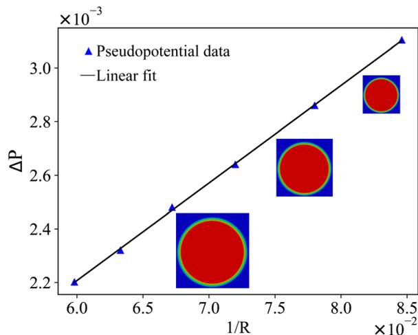
Fig. 13 Laplace test using the pseudopotential method at equilibrium for  $G_{k,1} = -7.9$ ,  $G_{k,2} = 4.9$  (see eqn (94)) and  $\tau_A = \tau_B = 1$ . From the linear fit we obtain the surface tension  $\Gamma = 0.00367$ . The images show the steady state of droplets as we vary the radius.
