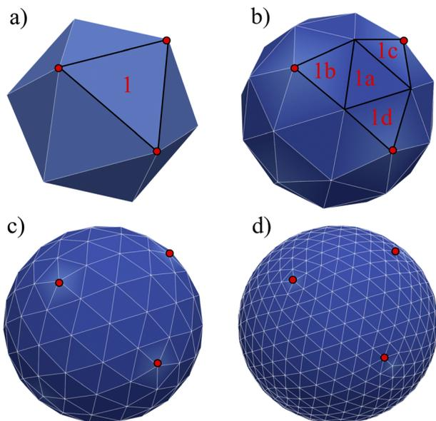
**Fig. 5** Loop subdivision mesh. The mesh is started from a solid such as an icosahedron (or other initial shapes such as a pyramid) which has 20 sides and 12 nodes. A triangular surface element is divided into 4. There are 3 levels of refinement shown: (a)–(d). For clarification, we highlight an initial triangle 1 which is divided into triangles 1a, 1b, 1c, and 1d. The red points just indicate the nodes of the initial face element.
