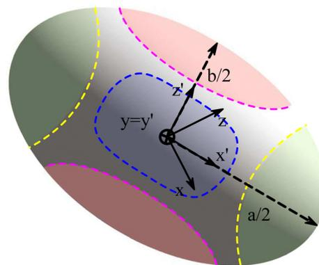
**Fig. 11** The final steady-state shape of droplet/capsule with the major axis,  $a$ , the minor axis of deformation,  $b$ , and the third axis,  $c$ . An additional reference frame  $(x', y', z')$  is defined, with the axes corresponding to the deformed droplet principal axes. The different regions of the droplet have been also highlighted for ease of reference: tips (green), belly (red) and sides (blue). Inspired by ref. 169.
