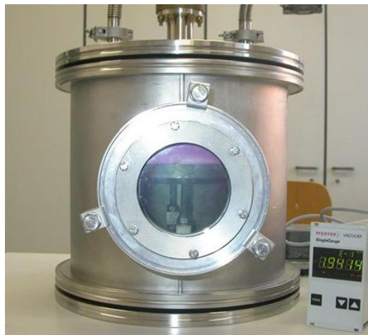
Fig. 1 The plasma chamber used in this work for the treatment of surfaces.
