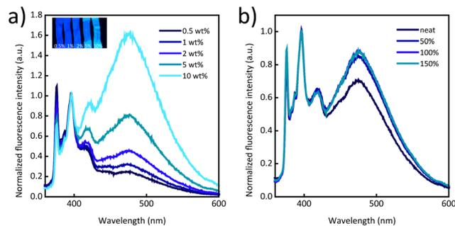
**Fig. 2** (a) Photoluminescence spectra of PI/Py-PEB blend films with a Py-PEB content of 0.5–10 wt%. The inset shows a picture of stretched films taken under illumination with 365 nm UV light. (b) Photoluminescence spectra of a PI/Py-PEB<sub>5</sub> film that was uniaxially deformed to the indicated strain. All spectra were acquired upon excitation at 310 nm and were normalized to the intensity of the monomer peak at 397 nm.
