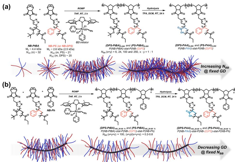
**Fig. 1** (a) ROMP of NB-*Pt*BA and NB-DPS/PS, and subsequent acid-catalyzed hydrolysis of *t*-BA repeating units. Illustrations of polymer shapes as a function of  $N_{BB}$ . (b) ROMP of NB-*Pt*BA, NB-DPS/PS, and NB-Ph, and subsequent acid-catalyzed hydrolysis of *t*-BA repeating units. Illustrations of polymer shapes as a function of GD. PS is shown as example in scheme.
