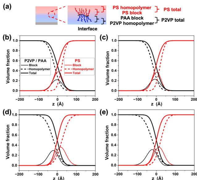
**Fig. 3** (a) Schematic illustration of a JBCP at polymer–polymer interface. Volume fraction profiles of different components at interfaces for JBCPs with variation of  $N_{BB}$ . (b)  $N_{BB} = 6$ , (c)  $N_{BB} = 24$ , (d)  $N_{BB} = 100$ , and (e)  $N_{BB} = 250$ .  $Z$  is the distance in Angstrom from the homopolymer interface. The legends for (c)–(e) are same as (b).
