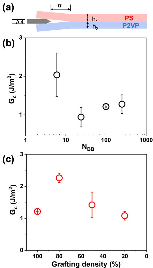
Fig. 9 Adhesion strength of JBCPs at homopolymer interface measured by asymmetric double cantilever beam (ADCB) test. (a) Scheme of ADCB test. Critical energy release rate ( $G_C$ ) as a function of (b)  $N_{BB}$  (grafting density = 100%) and (c) grafting density ( $N_{BB} = 100\%$ ).
