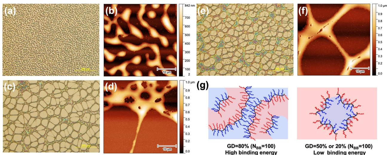
Fig. 8 Morphologies of thin film blends containing PS homopolymer and P2VP homopolymer (70 wt% to 30 wt%) with 10 wt% JBCP for different grafting densities at  $N_{BB} = 100$ . POM images of grafting density (a) 80%, (c) 50%, and (e) 20%. AFM images of (b) 80%, (d) 50%, and (f) 20%. (g) Schematic illustration of grafting density effect on binding energy at homopolymer interfaces. P2VP domain was washed by ethanol after thermal annealing of thin film blends.
