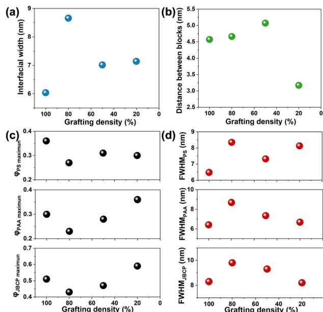
Fig. 6 Characteristics of segment density distributions for different grafting densities (GD) with  $N_{BB} = 100$ . (a) Interfacial width solved from PS||[(DPS-PAA)<sub>n</sub>||DP2VP]||Si. (b) Distance ( $d$ ) between two blocks (c) volume fraction maximum ( $\phi_{\text{maximum}}$ ) of PS block, PAA block and JBCP molecule. (d) Full-width half maximum (FWHM) of PS block, PAA block and JBCP molecule.
