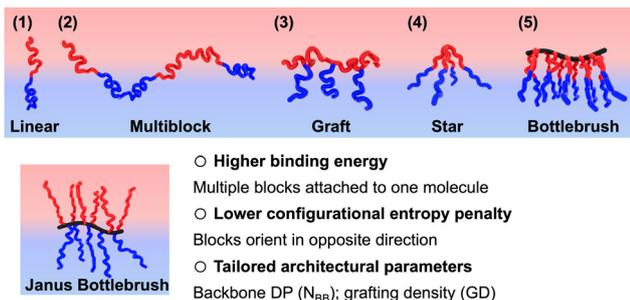
Scheme 1 Block copolymers (BCPs) as macromolecular compatibilizers.
