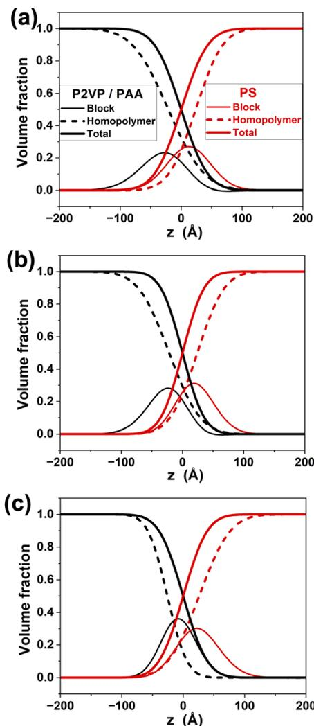
Fig. 5 Volume fraction profiles of different components at interfaces for JBCPs with  $N_{BB} = 100$  at different grafting densities of (a) 80%, (b) 50%, and (c) 20%.  $z$  is the distance from the homopolymer interface. The legends for (b) and (c) are same as (a).
