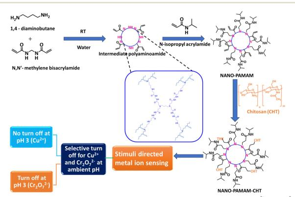
$\textbf{Scheme 1} \quad \text{Synthetic scheme for the NANO-PAMAM-CHT microgels and its application towards the selective detection of $Cu^{2+}$ and $Cr_2O_7^{2-}$ in water. }$
