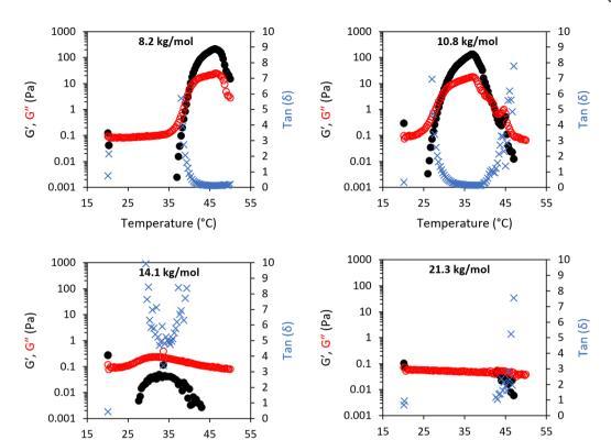
Fig. 3 SAOS temperature ramps of LAPONITE® and BCS composite fluids at 3 at 10 wt%, respectively. The effect of BCS molecular weight was explored (inset). G' and G'' are shown in black and red, respectively, with  $\tan\delta$  given in blue.
