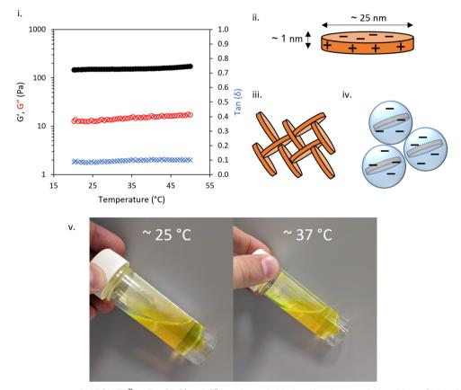
Fig. 2 (i) SAOS temperature ramps of LAPONITE $^{(8)}$  at 3 wt%. G' and G'' are shown in black and red, respectively, with  $an \delta$  given in blue. Rheological analysis conducted at 0.8 Pa and 6.283 rad s<sup>-1</sup>. (ii) schematic structure of LAPONITE® clay disks, with proposed "house of cards" (iii) and Wigner glass (iv) gel structures. (v) BCS 1 solution showing liquid-like behaviour at 25 and 37 °C. Fluorescein added for clarity of image
