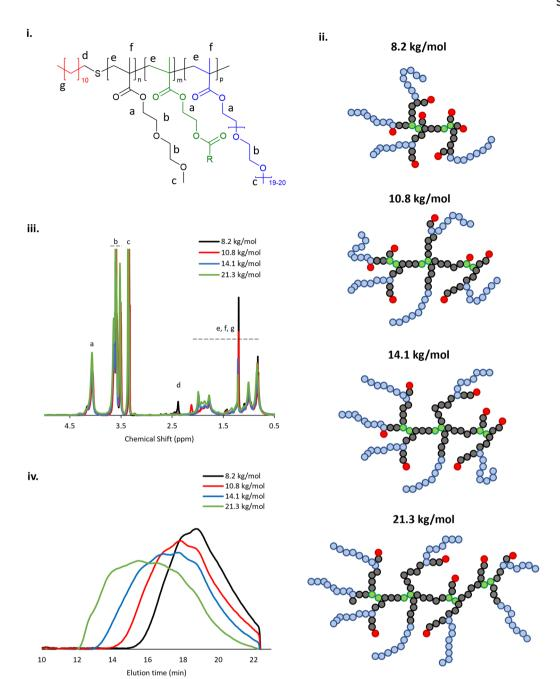
Fig. 1 (i) Simplified chemical structure of the BCS showing hydrophobic alkyl termini (red), thermoresponsive DEGMA (black), hydrophilic PEGMA (blue) and the cross-linking agent (EGDMA) used to induce branching (green). (ii)  $^{1}$ H NMR spectra of the four BCS with varied  $M_{n}$  and (iii) GPC chromatograms. (iv) Schematic representation of BCS showing increase in molecular weight and associated decrease in number of hydrophobic chain ends.
