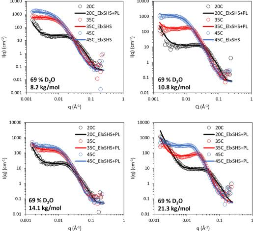
Fig. 6 SANS of 10 wt% BCS/3 wt% LAPONITE<sup>(B)</sup> clay in 69% v/v  $D_2O$  (in  $H_2O$ ), calculated to contrast match laponite. Lines represent a fit to the data shown as open circles, using the form factor inset. El: ellipsoid, SHS: sticky hard sphere, PL: power law. SANS data with error is included in Fig. S3-S6 (ESI†)
