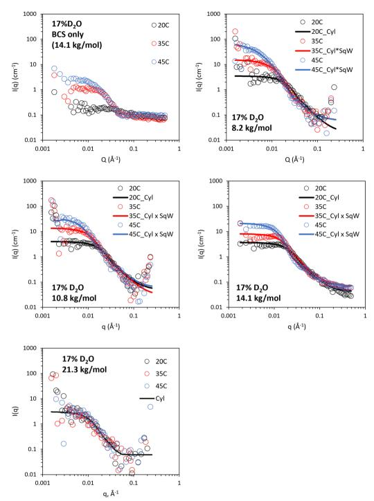
Fig. 8 SANS of 10 wt% BCS/3 wt% LAPONITE® clay in 17% v/v D<sub>2</sub>O (in H<sub>2</sub>O), calculated to contrast match PEGMA/DEGMA of BCS. Lines represent a fit to the data shown as open circles, using the form factor inset. Cyl: cylinder, SqW: square well. SANS data with error is included in Fig. S9-S12 (ESI†). Parameters from fitting are included in Tables S7-S9 (ESI†)
