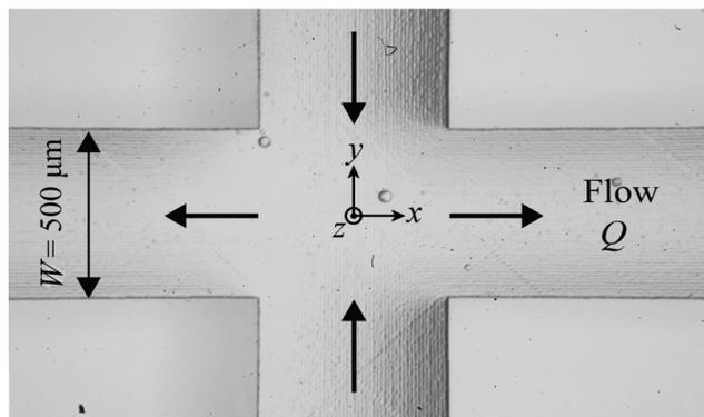
Fig. 1 Light micrograph of the cross-slot microchannel used in the present work. The width of each channel arm is  $W = 500 \mu\text{m}$  and the uniform height of the channel through  $z$  (into the page) is  $H = 2.0 \text{ mm}$ . The imposed volumetric flow rate through each of the four channel arms is denoted  $Q$ , with the direction indicated by arrows. The coordinate system, with origin at the center point of the geometry, is also shown.
