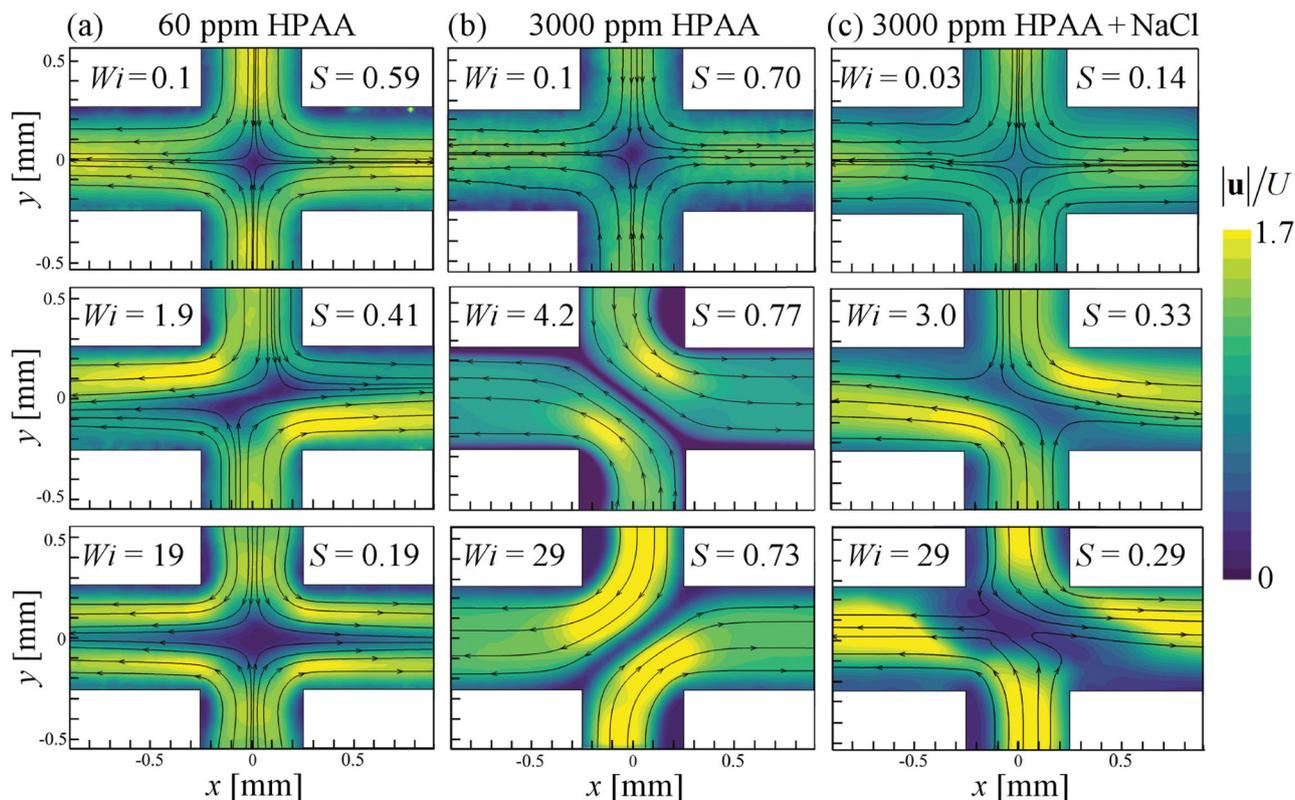
Fig. 5 Time-averaged velocity magnitude fields measured by microparticle image velocimetry with selected test solutions at the Weissenberg numbers and  $S$  values indicated, exemplifying the range of flow states observed experimentally. (a) 60 ppm HPAA without salt, (b) 3000 ppm HPAA without salt, (c) 3000 ppm HPAA with NaCl at  $0.5 \text{ mol L}^{-1}$ . Note that in all cases the flow is steady in time, except for in the bottom image of column (c).
