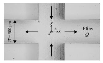
Fig. 1 Light micrograph of the cross-slot microchannel used in the present work. The width of each channel arm is  $W = 500 \mu m$  and the uniform height of the channel through z (into the page) is H = 2.0 mm. The imposed volumetric flow rate through each of the four channel arms is denoted Q, with the direction indicated by arrows. The coordinate system, with origin at the center point of the geometry, is also shown.
