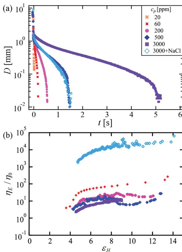
**Fig. 3** Characterization of the aqueous HPA test solutions in uniaxial extension in a CaBER device. (a) The filament diameter as a function of time from capillary thinning measurements made on all of the sample solutions. (b) The uniaxial extensional viscosity (scaled by the zero-shear-rate viscosity) as a function of the Hencky strain, determined within the exponentially-decaying region of the curves shown in part (a).
