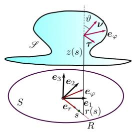
Fig. 3 Sketch of an axisymmetric  $nightcap \mathcal{S}$  obtained by deforming a flat disk S of radius R via the mapping  ${m y}$  described using (33). The unit vector  ${m
