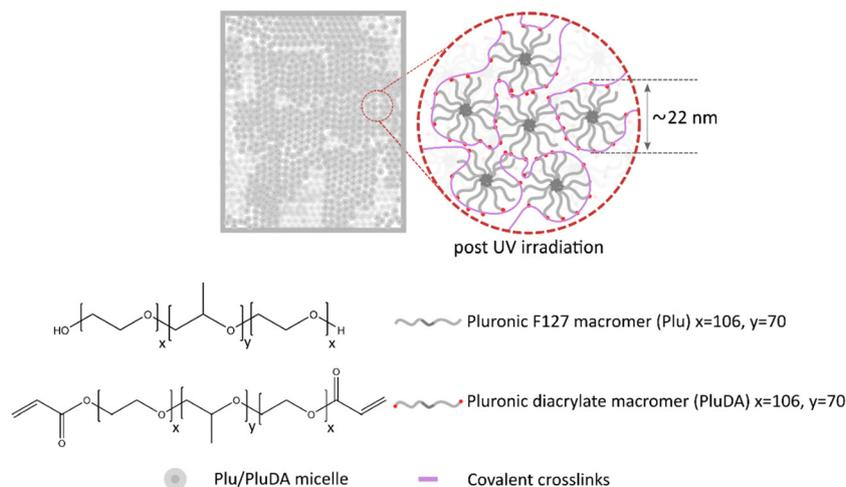
**Scheme 1** Micellar structure of the Plu/PluDA hydrogel representing the organization of the  $\text{PEO}_x\text{-PPO}_y\text{-PEO}_x$  triblock copolymer chains above the sol–gel transition temperature. The micelles have a diameter of ca. 22 nm and build aggregates that form a network with the inter- and intra-micellar covalent crosslinks between PluDA chains.
