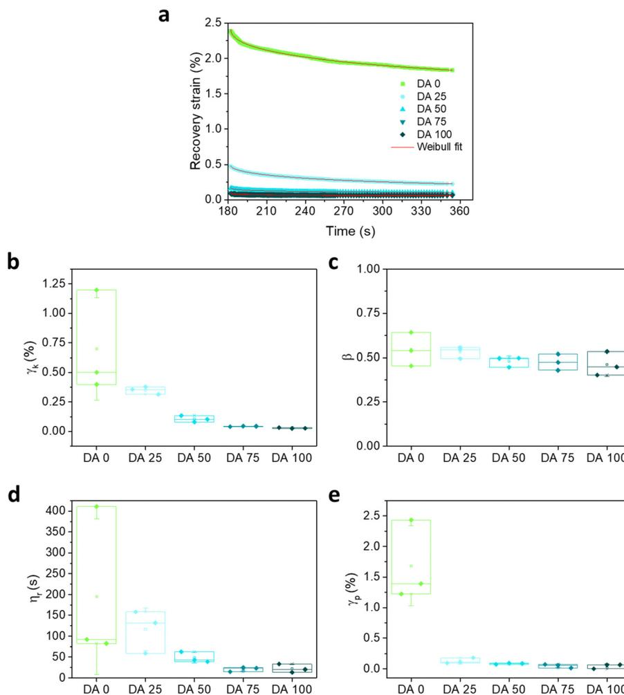
Fig. 5 (a) Recovery curves including fittings to the Weibull distribution function and (b)–(e) parameters of the Weibull fitting as function of DAX composition.  $N = 3$ , box represents 25 and 75 percentile values and whiskers indicate standard deviation.
