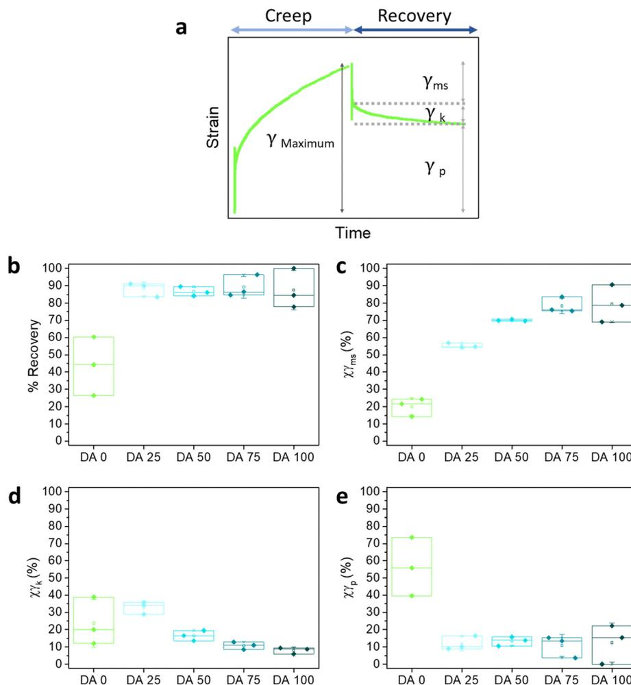
**Fig. 6** (a) Elastic, viscoelastic and plastic contributions obtained from the creep-recovery experiment. The curve corresponds to DA 0 at an applied stress of 100 Pa; (b) recovery (%) calculated from recovery curves at 180 s after 100 Pa applied stress; (c)–(e) contributions of elastic, (d) viscoelastic and (e) plastic deformation.  $N = 3$ , box represents 25 and 75 percentile values and whiskers indicate standard deviation.
