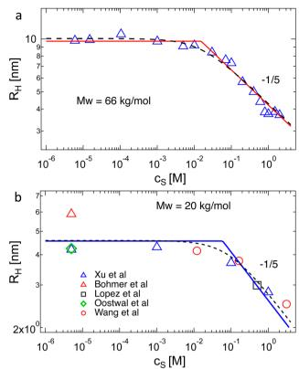
Fig. 31 Hydrodynamic radius of NaPSS in aqueous salt solutions at infinite dilution showing crossover between rod-like and flexible coil. Solid lines are fitted to  $R_{
