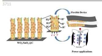
Synergistic effect of heterointerface engineering and oxygen vacancy in electro-spun polymer fibres derived carbon-supported 1D hierarchical WO<sub>3</sub>/ SnO<sub>2</sub> nanostructures for high-performance supercapacitor devices
