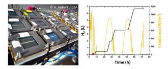
Thermally integrated photoelectrochemical devices with perovskite/silicon tandem solar cells: a modular approach for scalable direct water splitting
