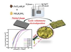
An iron phosphate hydroxide hydrate electrocatalyst: synergistic effects of Fe2+ and Fe3+ for enhanced hydrogen evolution reaction stability
