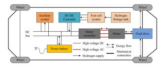
Design for six sigma-based energy management for a plug-in fuel cell electric bus considering the noise disturbance
