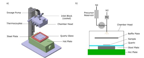
Fig. 1 (a) Technical drawing and (b) schematic of the APCVD system.
