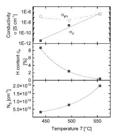
Fig. 5 Dark and photoconductivity  $\sigma_{\rm d}$  and  $\sigma_{\rm ph}$ , hydrogen content  $c_{\rm H}$ and spin density  $N_s$  of a-Si:H films deposited with pure trisilane as the precursor as a function of deposition temperature T. The lines are guides to the eye.
