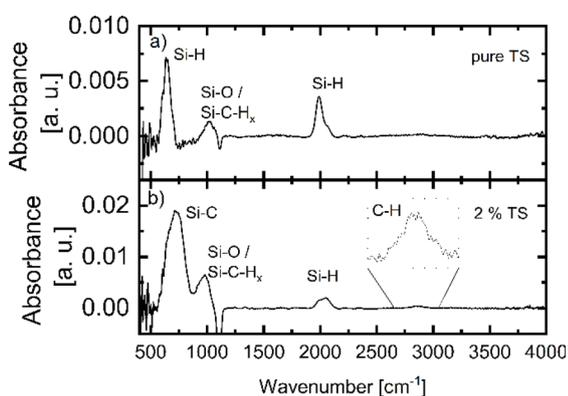
Fig. 7 FTIR spectra of (a) an a-Si:H film deposited at 440 °C with 20  $\mu$ l trisilane for 10 minutes and (b) an a-Si:H film deposited at 555 °C with 440  $\mu$ l of 2% trisilane diluted in cyclooctane for 10 minutes. The peaks are labeled with the corresponding bonds. In (b) the Si-H bending vibration peak at 640  $\text{cm}^{-1}$  is overlaid by the strong Si-C peak at around 720–780  $\text{cm}^{-1}$ .
