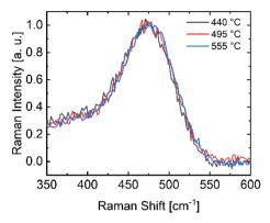
Fig. 4 Raman spectra showing the typical peak of Si-Si vibrations in amorphous silicon at 480 cm<sup>-1</sup> of a-Si:H films deposited at 440, 495 and 555 °C.
