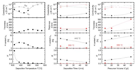
Fig. 2 Dark and photoconductivity  $\sigma_d$  and  $\sigma_{ph}$ , thickness d, hydrogen content  $c_H$  and microstructure parameter R of a-Si:H films deposited with pure trisilane as a precursor as a function of (a) deposition temperature T, (b) deposition time t, and (c) precursor volume V. t and V were varied at temperatures T = 440 °C (gray) and 555 °C (red). The lines are guides to the eye.
