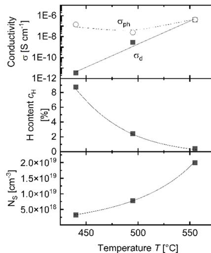
Fig. 5 Dark and photoconductivity  $\sigma_{\text{d}}$  and  $\sigma_{\text{ph}}$ , hydrogen content  $c_{\text{H}}$  and spin density  $N_{\text{s}}$  of a-Si:H films deposited with pure trisilane as the precursor as a function of deposition temperature  $T$ . The lines are guides to the eye.
