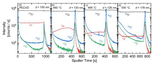
Fig. 6 Silicon, hydrogen, carbon, and oxygen SIMS profiles of (a) an intrinsic PECVD film and APCVD films deposited at (b) 440 °C, (c) 495 °C and (d) 555 °C.
