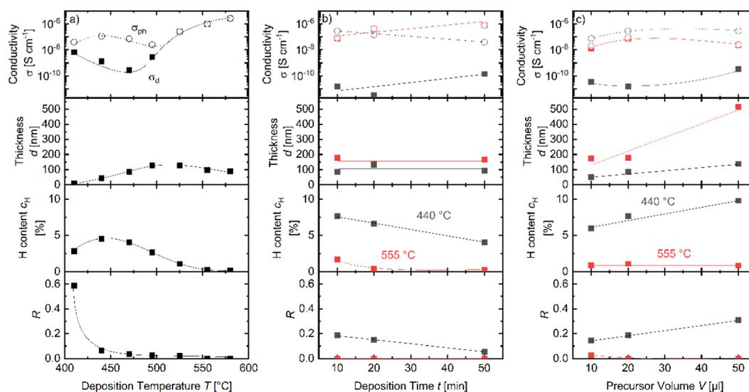
Fig. 2 Dark and photoconductivity  $\sigma_d$  and  $\sigma_{ph}$ , thickness  $d$ , hydrogen content  $c_H$  and microstructure parameter  $R$  of a-Si:H films deposited with pure trisilane as a precursor as a function of (a) deposition temperature  $T$ , (b) deposition time  $t$ , and (c) precursor volume  $V$ .  $t$  and  $V$  were varied at temperatures  $T = 440 \text{ }^\circ\text{C}$  (gray) and  $555 \text{ }^\circ\text{C}$  (red). The lines are guides to the eye.
