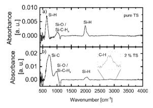
Fig. 7 FTIR spectra of (a) an a-Si:H film deposited at 440 °C with 20  $\mu$ l trisilane for 10 minutes and (b) an a-Si:H film deposited at 555 °C with 440  $\mu$ l of 2% trisilane diluted in cyclooctane for 10 minutes. The peaks are labeled with the corresponding bonds. In (b) the Si–H bending vibration peak at 640 cm $^{-1}$  is overlaid by the strong Si–C peak at around 720–780 cm $^{-1}$ .
