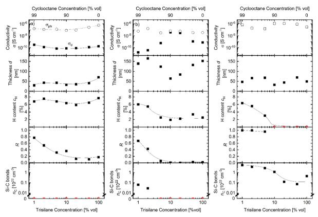
Fig. 8 Dark and photoconductivity  $\sigma_d$  and  $\sigma_{ph}$ , thickness d, hydrogen content  $c_H$ , microstructure parameter R and the amount of Si–C bonds  $n_c$ of a-Si:H films as a function of the trisilane concentration within the precursor deposited at a deposition temperature T of (a) 440 °C, (b) 495 °C and (c) 555 °C. The red marked points were set to 0, since the signal-to-noise ratio was too small to determine a peak within the FTIR spectrum. The lines are guides to the eye.
