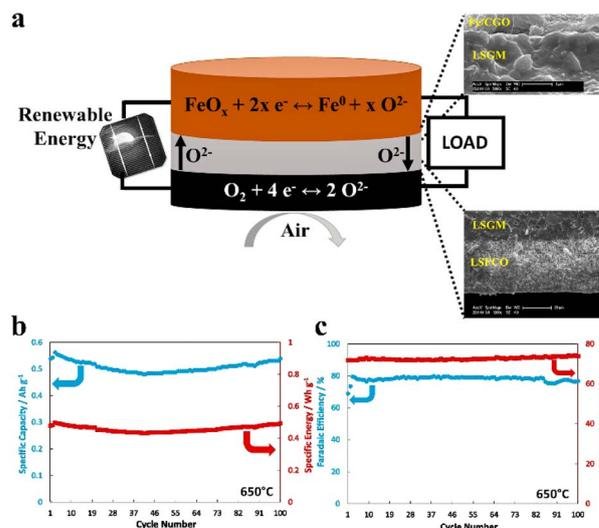
Fig. 8 (a) Configuration and SEM images of the interfaces in the ceramic iron–air battery.<sup>150</sup> (b) Specific capacity and specific energy of the ceramic IAB at 650 °C.<sup>150</sup> (c) Faradaic efficiency and voltage efficiency of the ceramic IAB versus the number of cycles at 650 °C.<sup>150</sup>
