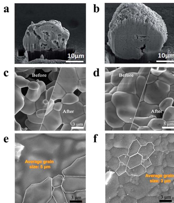
Fig. 11 SEM images of the cross-section of an iron particle before (a) and after oxidation (b).<sup>173</sup> Comparison of SEM images of Fe<sub>2</sub>O<sub>3</sub> (c) and 1% Cu-doped Fe<sub>2</sub>O<sub>3</sub> (d) before and after redox reactions.<sup>174</sup> Comparison of SEM images of Fe<sub>2</sub>O<sub>3</sub> (e) and La-doped Fe<sub>2</sub>O<sub>3</sub> (f) before and after redox reactions.<sup>175</sup>
