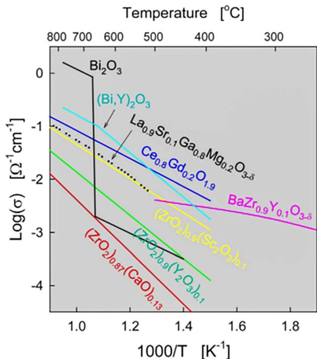
Fig. 10 Ionic conductivities of solid-oxide electrolytes.<sup>161</sup>
