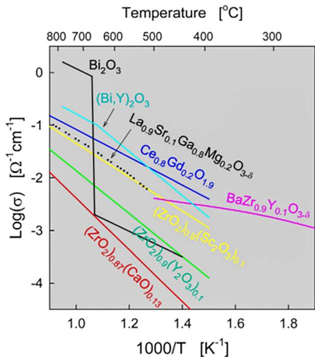
Fig. 10 Ionic conductivities of solid-oxide electrolytes.<sup>161</sup>
