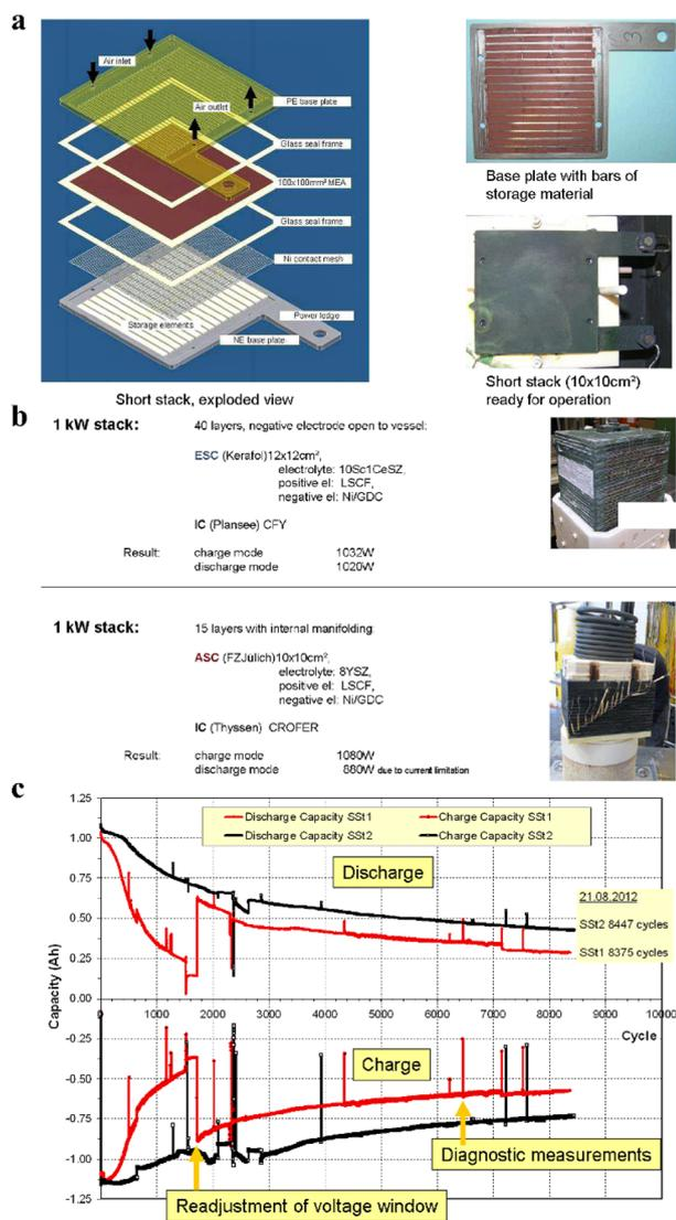
Fig. 6 (a) Short stack arrangement of the SOIARB energy storage system.<sup>136</sup> (b) Laboratory tests of the 1 kW SOIARB stack.<sup>136</sup> (c) Storage capacity degradation rates of the SOIARB system.<sup>136</sup>
