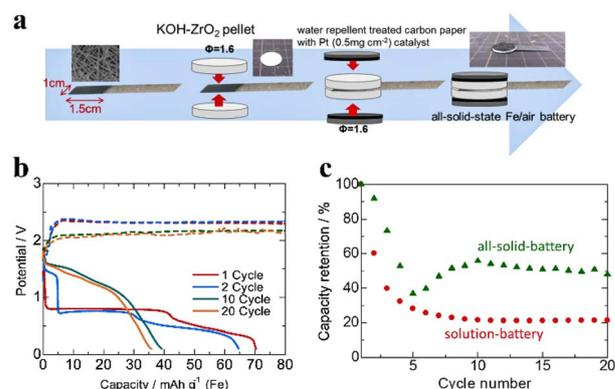
Fig. 3 (a) Assembly steps of a room-temperature all-solid iron–air battery.<sup>89</sup> (b) Charge–discharge curves of a room-temperature all-solid iron–air battery.<sup>89</sup> (c) Comparison of the capacity retention between an aqueous iron–air battery and room-temperature all-solid iron–air battery.<sup>89</sup>
