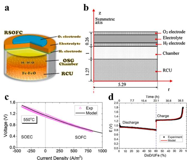
Fig. 5 (a) Schematic of the SOIARB configuration.<sup>131</sup> (b) The finite element method model of the SOIARB (unit: mm).<sup>131</sup> (c) Validation of the *V–I* curve at 550 °C.<sup>131</sup> (d) Validation of the *E* vs. Fe-utilization curve.<sup>131</sup>
