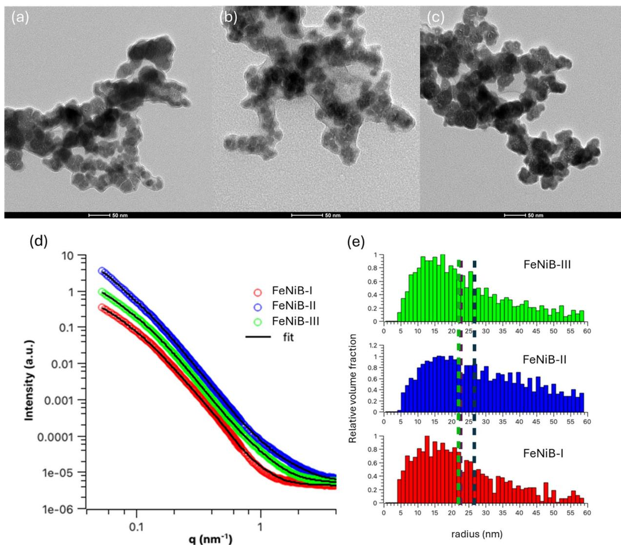
Fig. 2 Morphological observations and size distribution analysis. TEM micrographs of (a) FeNiB-I, (b) FeNiB-II, (c) FeNiB-III, (d) SAXS patterns of the electrocatalyst powders, and (e) their corresponding volume-weighted particle size distributions, as determined by SAXS. The vertical dashed lines indicate the mean value of the radius distributions.
