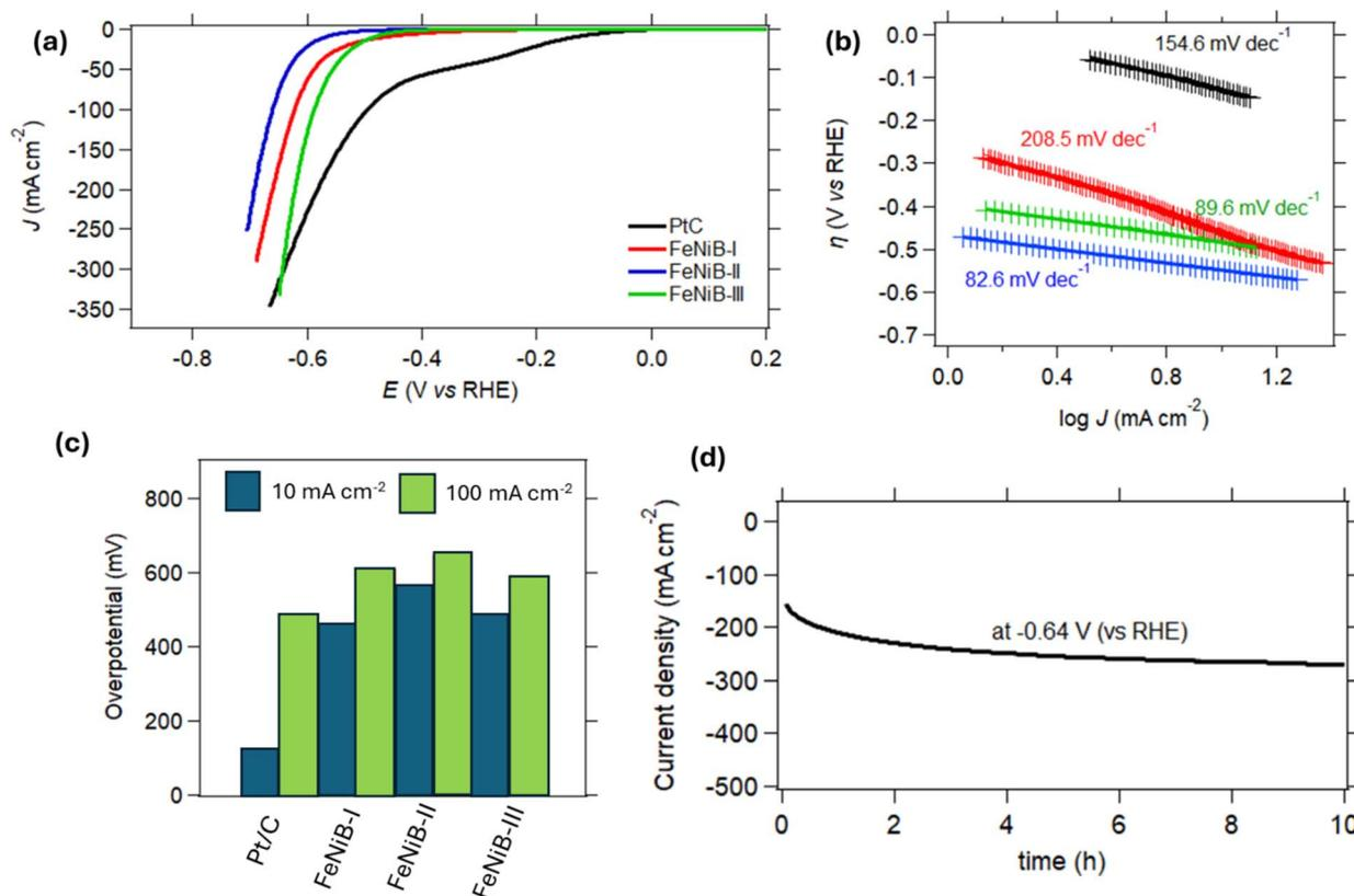
Fig. 8 HER performance of the electrocatalyst powders. (a) Polarization curves, (b) Tafel slopes, (c) overpotentials at 10 and 100 mA cm<sup>-2</sup>, (d) chronoamperometric curve of FeNiB-I at -0.64 V (vs. RHE) for 10 h.
