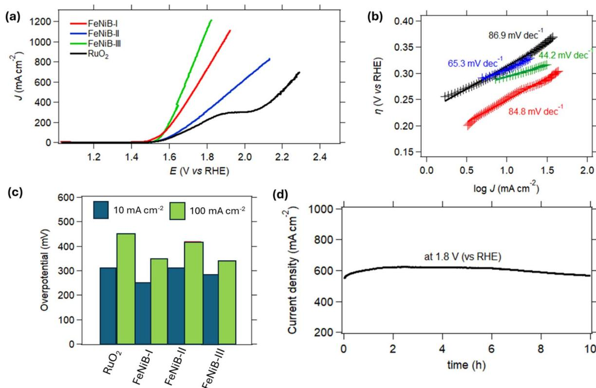
Fig. 7 OER performance of the electrocatalyst powders. (a) Polarization curves, (b) Tafel slopes, (c) overpotentials at 10 and 100 mA cm<sup>-2</sup>, (d) chronoamperometric curve of FeNiB-III at 1.8 V (vs. RHE) for 10 h.
