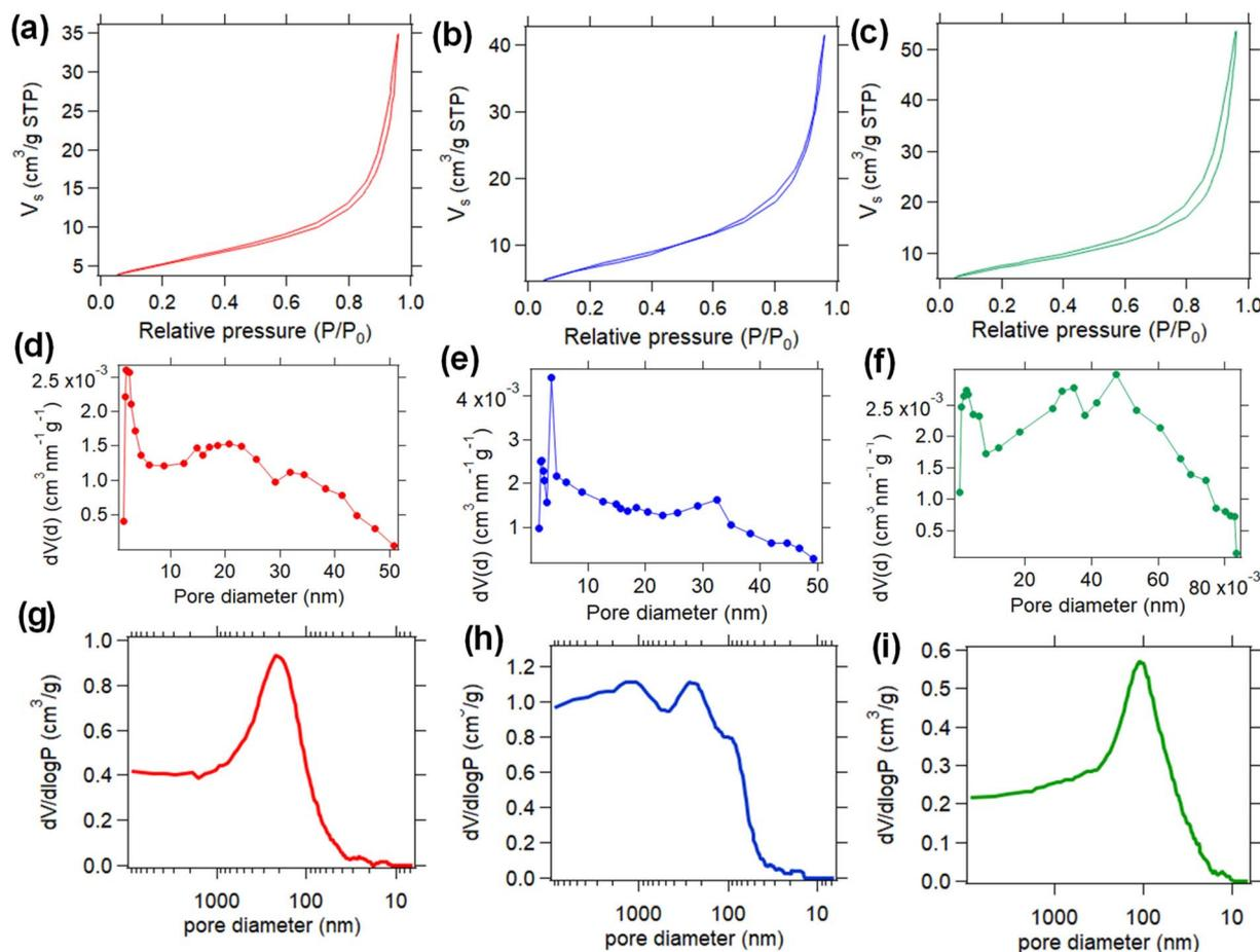
Fig. 4 Nitrogen adsorption–desorption isotherms for (a) FeNiB-I, (b) FeNiB-II, and (c) FeNiB-III, BJH pore size distributions for (d) FeNiB-I, (e) FeNiB-II, and (f) FeNiB-III, and pore surface area distribution curves, with cumulative surface area overlaid (obtained from Hg porosimetry) for (g) FeNiB-I, (h) FeNiB-II, and (i) FeNiB-III.
