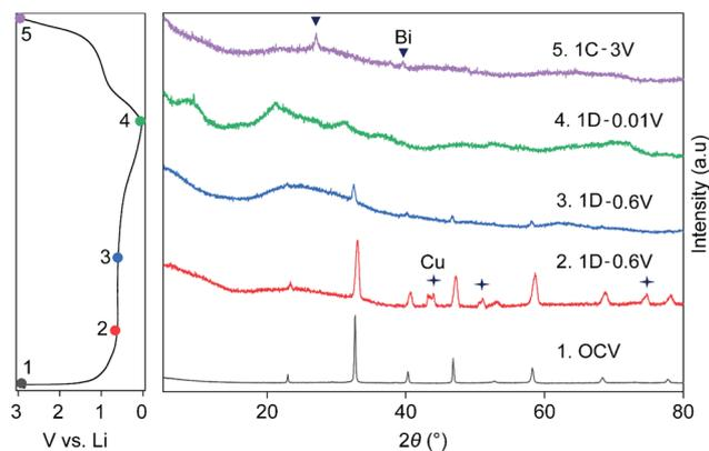
Fig. 4 *Ex situ* XRD analysis of the perovskite NBT anode after lithium (de)insertion, taken at the following points: (1) OCV (black); (2) first discharge to  $0.6 \text{ V}$  at the start of conversion (red); (3) first discharge to  $0.6 \text{ V}$  at the end of the conversion step (blue); (4) full first discharge to  $0.01 \text{ V}$  (green); (5) full charge to  $3.0 \text{ V}$  (lavender).
