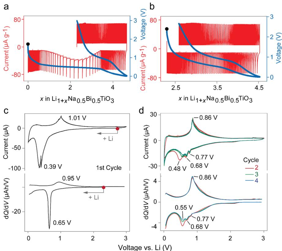
Fig. 3 Comparison of Li insertion in perovskite NBT in the first and subsequent cycles. PITT curves for the (a) first and (b) second cycle. CV and  $dQ/dV$  curves, at  $0.01 \text{ V s}^{-1}$  and  $10 \text{ mA g}^{-1}$  respectively, of the (c) first cycle, and (d) second, third and fourth cycles. The voltage window was fixed at  $0.01\text{--}3 \text{ V}$  (vs. Li) for these Li-NBT half-cells.
