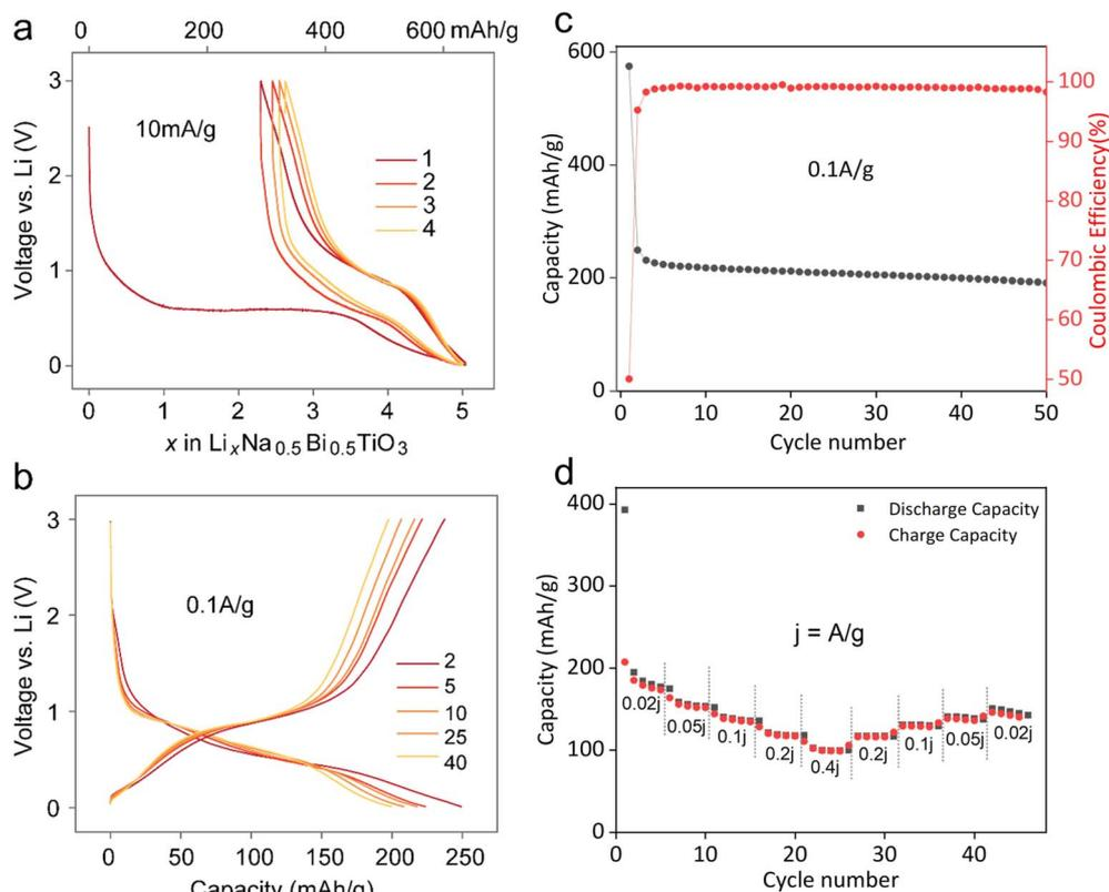
Fig. 2 Electrochemical performance of lithium insertion in the NBT perovskite. Galvanostatic voltage profiles at (a) slow  $10 \text{ mA g}^{-1}$  and (b) fast  $0.1 \text{ A g}^{-1}$  current densities, (c) cycle life, and (d) rate performance of Li-NBT half cells.
