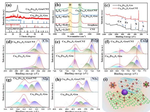
Fig. 2 XRD (a), Raman spectra (b) and XPS spectra (c) of  $\text{Co}_{0.2}\text{Fe}_{0.6}\text{S}_x\text{-Gra/CNT}$ ; XPS spectra of C 1s (d), Fe 2p (e), Co 2p (f), S 2p (g), and N 1s (h). (i) The electronic structure schematic illustration of  $\text{Co}_{0.2}\text{Fe}_{0.6}\text{S}_x\text{-Gra/CNT}$ .
