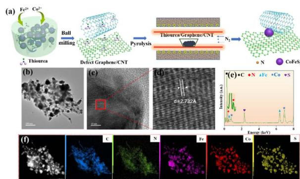
Fig. 1 (a) Schematic illustration of the synthesis of  $\text{CoFeS}_x\text{-Gra/CNT}$ ; (b) TEM (c and d) HRTEM images and (e) EDS of  $\text{Co}_{0.2}\text{Fe}_{0.6}\text{S}_x\text{-Gra/CNT}$ ; (f) element mappings of the NSP-Gra.
