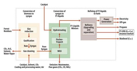
Fig. 2 System boundary for the cradle-to-gate life-cycle assessment of sustainable aviation fuel (SAF) production from forest residues.
