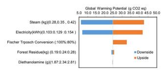
Fig. 8 Sensitivity analysis of the global warming impact of SAF production from forest residues.
