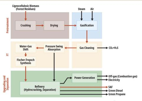
Fig. 1 Overview of the gasification-Fischer-Tropsch process for SAF production from forest residues<sup>62</sup> (main product process flow in red and byproducts and emission in black).
