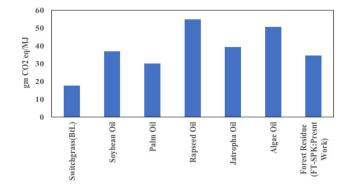
Fig. 7 Comparative global warming impact of SAF from different feedstocks
