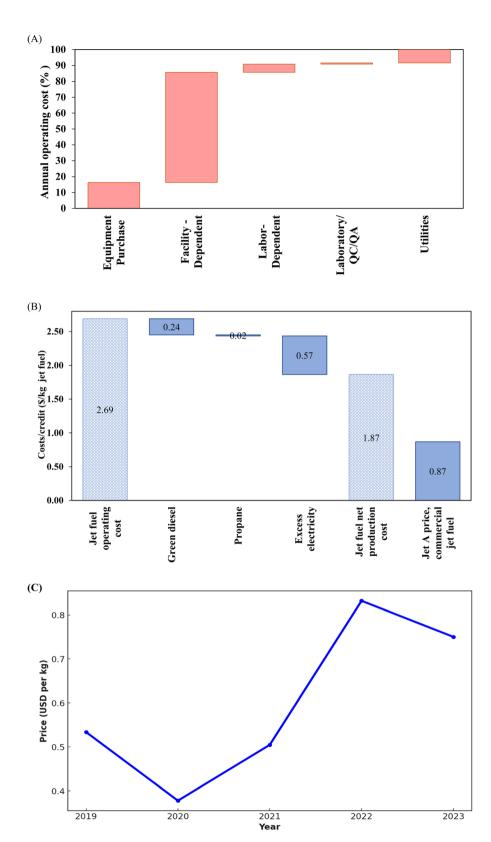
Fig. 4 (A) Operating cost and (B) minimum selling price of sustainable aviation fuel (SAF) production from forest residues and (C) historical price fluctuation of commercial jet fuel.
