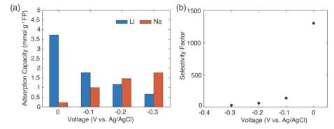
Fig. 9 Electrochemical reduction of FP to capture cations from a brine solution containing Li<sup>+</sup>: Na<sup>+</sup> molar ratio of 1:78. (a) The cations adsorption capacity of the working electrode (FP) and (b) the selectivity factor  $\alpha_{Na}^{Va}$  for FP was assessed after 50% extent of reduction of the FP at constant voltages of 0, -0.1, -0.2, and -0.3 V (vs. Ag/AgCl).
