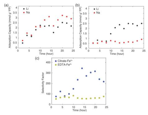
Fig. 5 Li<sup>+</sup> (black circles) and Na<sup>+</sup> (red circles) adsorption capacity as a function of time for extraction of Li<sup>+</sup> from 1:78 Li<sup>+</sup>: Na<sup>+</sup> brine using (a) EDTA-Fe<sup>2+</sup> and (b) citrate-Fe<sup>2+</sup>. The extraction experiments were conducted at 45 °C. (c) Selectivity factors ( $\alpha_{Na}^{Li}$ ) for Li<sup>+</sup> extraction from EDTA-Fe<sup>2+</sup> (yellow-green circles) and citrate-Fe<sup>2+</sup> (blue circles)
