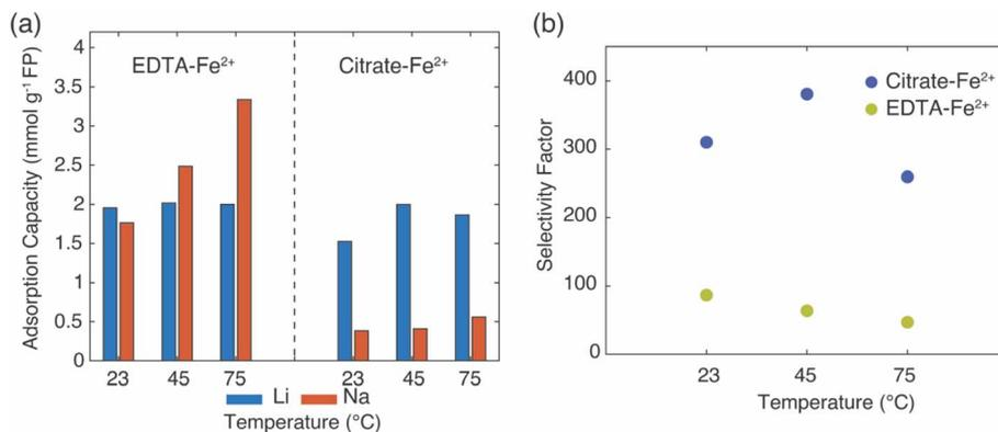
Fig. 10 (a) Adsorption capacities for Li<sup>+</sup> and Na<sup>+</sup> and (b) selectivity factors  $\alpha_{\text{Na}}^{\text{Li}}$  in FP from brine that more closely simulated Salton Sea brine (more specific composition in Table S3†). Cation uptake was driven by the redox mediator indicated on the figure.
