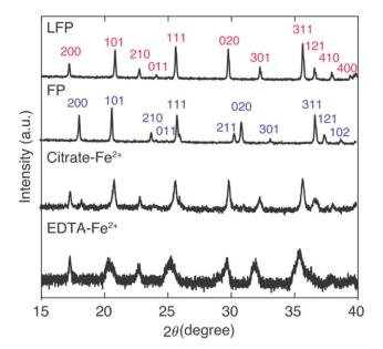
Fig. 4 XRD patterns for the as-received LFP powder, FP after chemical oxidation of the LFP, and chemically reduced FP after contact with brine containing citrate-Fe<sup>2+</sup> mediator and EDTA-Fe<sup>2+</sup> mediator, respectively. The mediator concentration was 0.1 M and the brine had 1:78 Li<sup>+</sup>: Na<sup>+</sup> stoichiometry. The brine reaction was at 45 °C for a duration of 24 hours. Indexes were assigned based on PDF-01-078-7908 for LFP and PDF-04-017-0610 for FP.28
