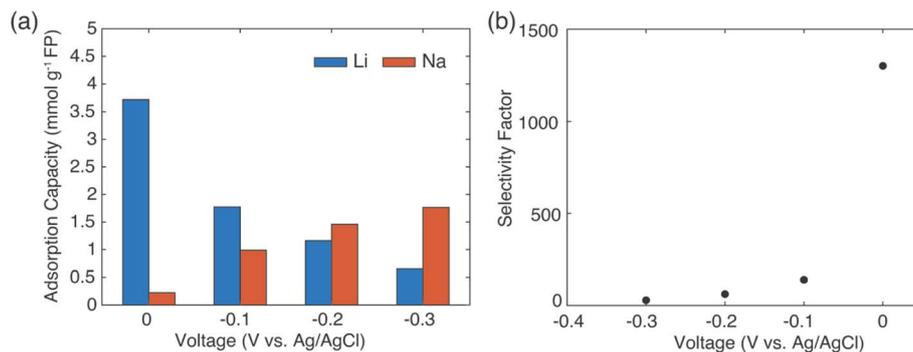
Fig. 9 Electrochemical reduction of FP to capture cations from a brine solution containing Li<sup>+</sup> : Na<sup>+</sup> molar ratio of 1 : 78. (a) The cations adsorption capacity of the working electrode (FP) and (b) the selectivity factor  $\alpha_{\text{Na}}^{\text{Li}}$  for FP was assessed after 50% extent of reduction of the FP at constant voltages of 0, -0.1, -0.2, and -0.3 V (vs. Ag/AgCl).
