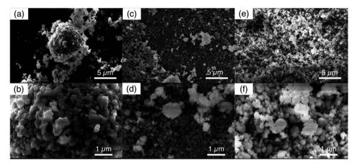
Fig. 7 SEM images of (a and b) the initial FP prepared by chemical oxidation, (c and d) FP after 5 cycles of Li<sup>+</sup> extraction/release using redox mediator EDTA-Fe<sup>2+</sup>, and (e and f) FP after 5 cycles of Li<sup>+</sup> extraction/release using redox mediator citrate-EDTA-Fe<sup>2+</sup>. Scale bars indicated in the images, where the top row is at relatively lower magnification relative to the bottom row of images.
