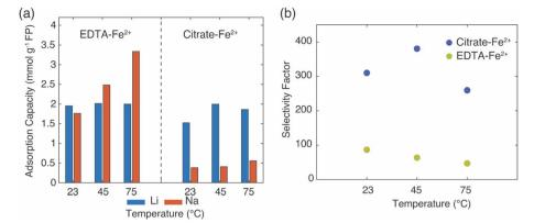
Fig. 10 (a) Adsorption capacities for Li<sup>+</sup> and Na<sup>+</sup> and (b) selectivity factors  $\alpha_{Na}^{Li}$  in FP from brine that more closely simulated Salton Sea brine (more specific composition in Table S3†). Cation uptake was driven by the redox mediator indicated on the figure.
