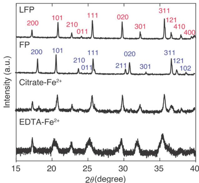
Fig. 4 XRD patterns for the as-received LFP powder, FP after chemical oxidation of the LFP, and chemically reduced FP after contact with brine containing citrate-Fe<sup>2+</sup> mediator and EDTA-Fe<sup>2+</sup> mediator, respectively. The mediator concentration was 0.1 M and the brine had 1 : 78 Li<sup>+</sup> : Na<sup>+</sup> stoichiometry. The brine reaction was at 45 °C for a duration of 24 hours. Indexes were assigned based on PDF-01-078-7908 for LFP and PDF-04-017-0610 for FP.<sup>28</sup>
