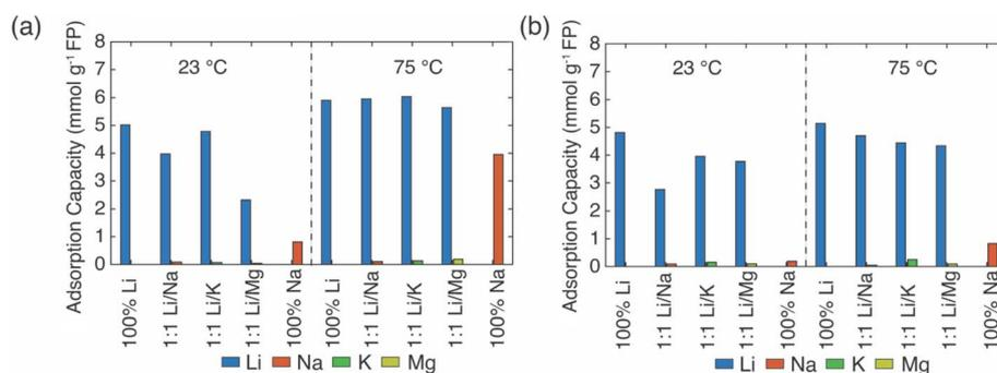
Fig. 2 Cation uptake (adsorption capacity) from chemical reduction of FP using brines containing redox mediators. The redox mediators were (a) EDTA-Fe<sup>2+</sup> and (b) citrate-Fe<sup>2+</sup>. All the salts were alkali metal chlorides, with each monovalent cation concentration of ~1 M in the mixed salt solution. The two temperatures of the chemical redox reaction were 23 °C and 75 °C, with the relevant condition of the reaction indicated on the figure.
