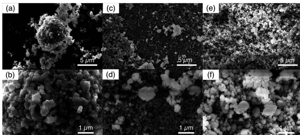
Fig. 7 SEM images of (a and b) the initial FP prepared by chemical oxidation, (c and d) FP after 5 cycles of Li<sup>+</sup> extraction/release using redox mediator EDTA-Fe<sup>2+</sup>, and (e and f) FP after 5 cycles of Li<sup>+</sup> extraction/release using redox mediator citrate-EDTA-Fe<sup>2+</sup>. Scale bars indicated in the images, where the top row is at relatively lower magnification relative to the bottom row of images.
