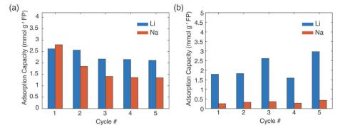
Fig. 6 Li<sup>+</sup> and Na<sup>+</sup> uptake into FP during multiple cycles of cation release via chemical oxidation of the powder and cation insertion via chemical reduction in brine with mediators (a) EDTA-Fe<sup>2+</sup> and (b) citrate-Fe<sup>2+</sup>
