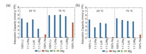
Fig. 2 Cation uptake (adsorption capacity) from chemical reduction of FP using brines containing redox mediators. The redox mediators were (a) EDTA-Fe<sup>2+</sup> and (b) citrate-Fe<sup>2+</sup>. All the salts were alkali metal chlorides, with each monovalent cation concentration of  $\sim$ 1 M in the mixed salt solution. The two temperatures of the chemical redox reaction were 23 °C and 75 °C, with the relevant condition of the reaction indicated on the figure.
