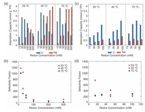
Fig. 3 (a) Uptake of Li<sup>+</sup> and Na<sup>+</sup> and (b)  $\alpha_{\rm ha}^{\rm Li}$  and reduction of FP with redox mediators EDTA-Fe<sup>2+</sup>. (c) Uptake of Li<sup>+</sup> and Na<sup>+</sup> and (d)  $\alpha_{Na}^{\parallel j}$  after reduction by citrate – Fe<sup>2+</sup>. The mediator concentration and reduction temperatures are indicated on the figure. The surrounding brine had a 1:78 Li<sup>+</sup>: Na<sup>+</sup> molar concentration.
