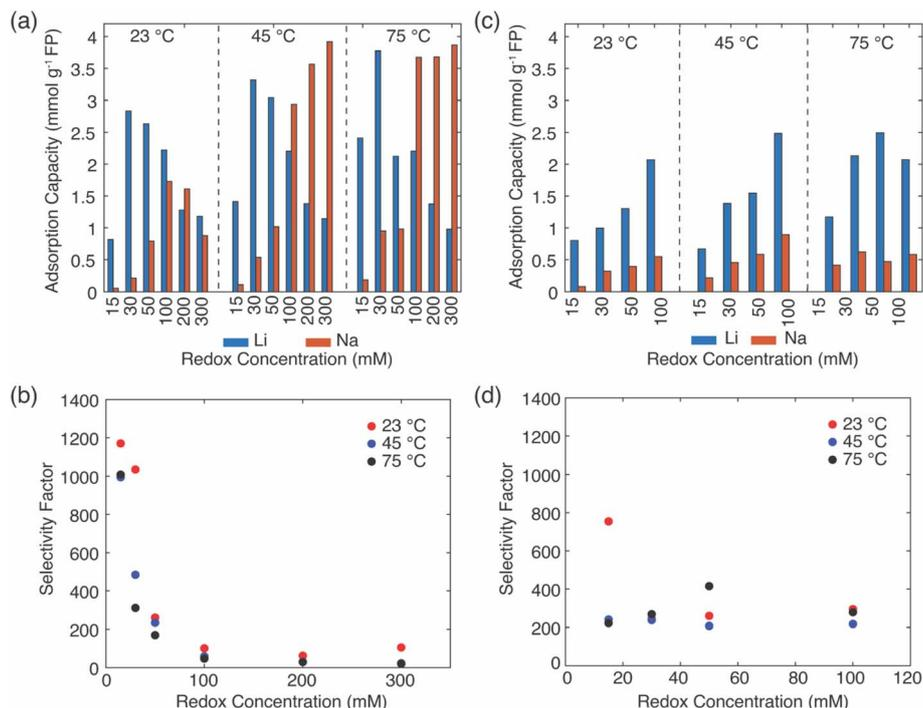
**Fig. 3** (a) Uptake of  $\text{Li}^+$  and  $\text{Na}^+$  and (b)  $\alpha_{\text{Na}}^{\text{Li}}$  during chemical reduction of FP with redox mediators EDTA- $\text{Fe}^{2+}$ . (c) Uptake of  $\text{Li}^+$  and  $\text{Na}^+$  and (d)  $\alpha_{\text{Na}}^{\text{Li}}$  after reduction by citrate- $\text{Fe}^{2+}$ . The mediator concentration and reduction temperatures are indicated on the figure. The surrounding brine had a 1 : 78  $\text{Li}^+$  :  $\text{Na}^+$  molar concentration.
