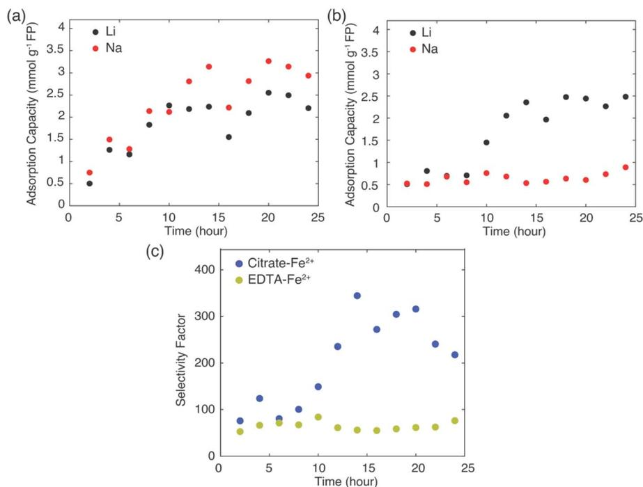
Fig. 5 Li<sup>+</sup> (black circles) and Na<sup>+</sup> (red circles) adsorption capacity as a function of time for extraction of Li<sup>+</sup> from 1 : 78 Li<sup>+</sup> : Na<sup>+</sup> brine using (a) EDTA-Fe<sup>2+</sup> and (b) citrate-Fe<sup>2+</sup>. The extraction experiments were conducted at 45 °C. (c) Selectivity factors ( $\alpha_{\text{Na}}^{\text{Li}}$ ) for Li<sup>+</sup> extraction from EDTA-Fe<sup>2+</sup> (yellow-green circles) and citrate-Fe<sup>2+</sup> (blue circles).
