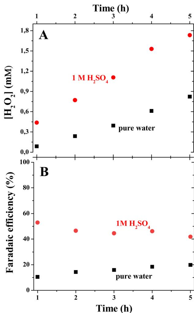
Fig. 2  $\text{H}_2\text{O}_2$  electrosynthesis at the cathode. The time dependencies of  $\text{H}_2\text{O}_2$  concentration (A) and faradaic efficiency (B) of  $\text{H}_2\text{O}_2$  electrosynthesis in pure water and 1 M  $\text{H}_2\text{SO}_4$ .
