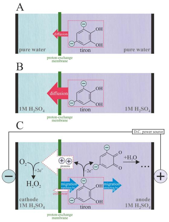
Scheme 1 Processes occurring in the electrolyzer under zero current ((A) pure water; (B) 1 M H<sub>2</sub>SO<sub>4</sub>) and non-zero current (C) conditions.
