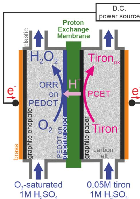
Scheme 2 Membrane electrolyzer based on the proton-exchange membrane.
