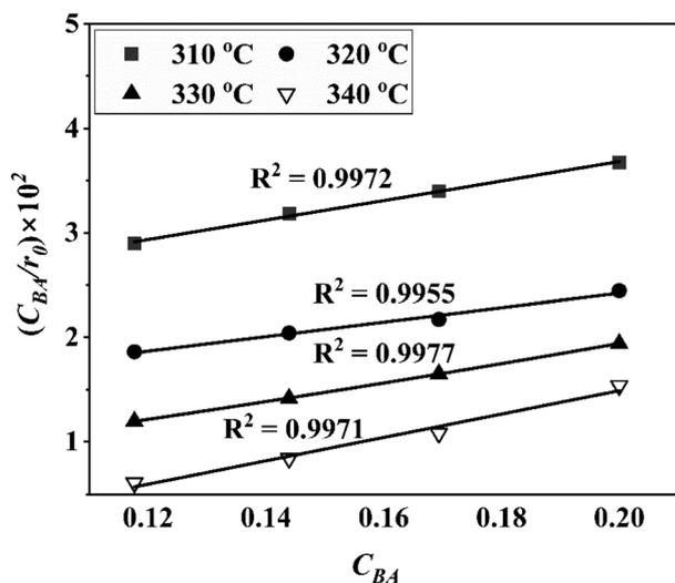
Fig. 6 Plot of the linearised form of the best fitted kinetic models (I) dual sites adsorption of dissociatively adsorbed H<sub>2</sub> and (II) dual sites adsorption of non-dissociatively adsorbed H<sub>2</sub>.
