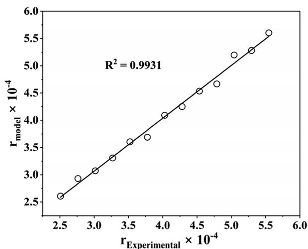
Fig. 7 Parity plot for the best fitted kinetic model (dual sites adsorption of dissociatively adsorbed H<sub>2</sub>).
