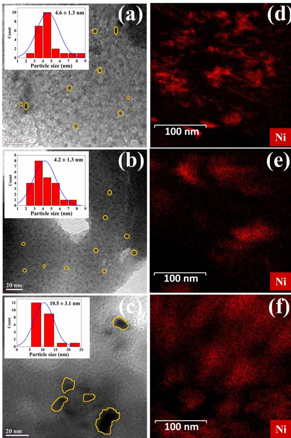
Fig. 1 TEM image of the prepared catalysts; (a) m-Ni/ZSM-5, (b) h-Ni/ZSM-5, and (c) Ni/SiO<sub>2</sub>. Elemental mapping by dark-field scanning TEM; (d) m-Ni/ZSM-5, (e) h-Ni/ZSM-5, and (f) Ni/SiO<sub>2</sub>.
