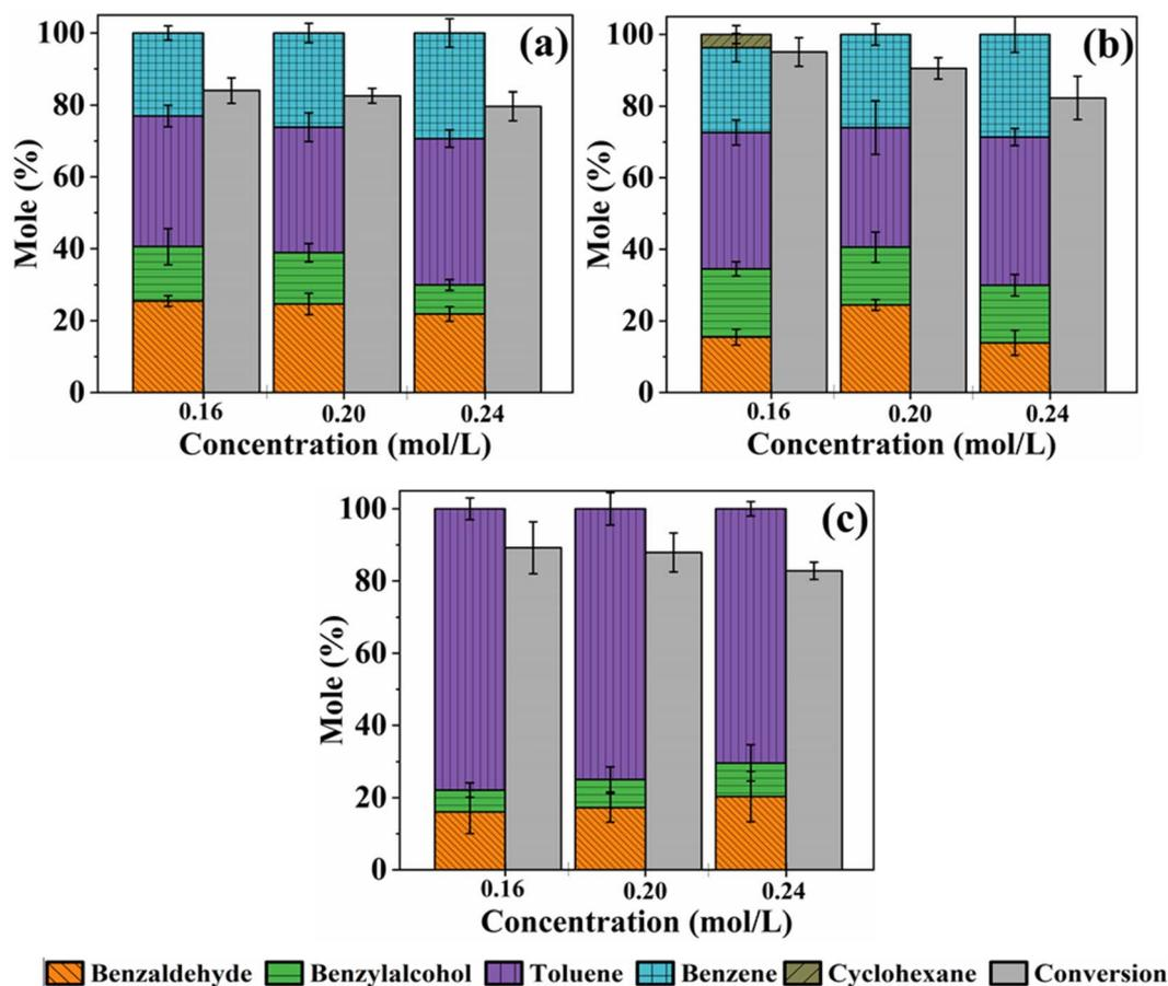
Fig. 4 Conversion and product distribution as a function of initial concentration during the HDO reaction of benzoic acid over m-Ni/ZSM-5 (a), h-Ni/ZSM-5 (b), and Ni/SiO<sub>2</sub> (c). Catalyst loading; 100 mg, reaction temperature; 330 °C, solvent; tetralin, benzoic acid initial concentration; 0.16 – 0.24 M, reaction time; 6 hours.
