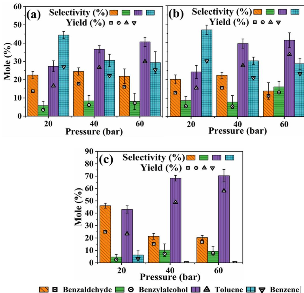
Fig. 3 Influence of H<sub>2</sub> pressure on product distribution during the HDO of benzoic acid over m-Ni/ZSM-5 (a), h-Ni/ZSM-5 (b), and Ni/SiO<sub>2</sub> (c). Catalyst loading; 100 mg, reaction temperature; 330 °C, solvent; tetralin, benzoic acid initial concentration; 0.24 M, reaction time; 6 hours.
