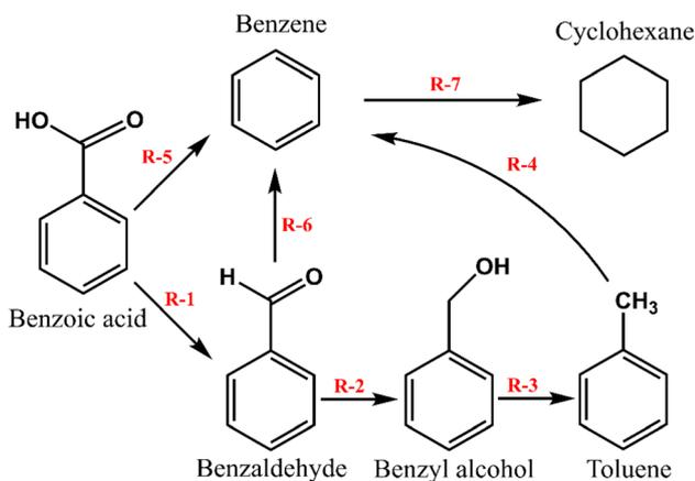
Fig. 2 Simplified reaction pathway for the benzoic acid transformation over m-Ni/ZSM-5, h-Ni/ZSM-5, and Ni/SiO<sub>2</sub> catalysts. (R-1; Deoxygenation, R-2; hydrogenation, R-3; deoxygenation, R-4; demethylation, R-5; decarboxylation, R-6; decarbonylation, R-7; hydrogenation).<sup>60,77</sup>
