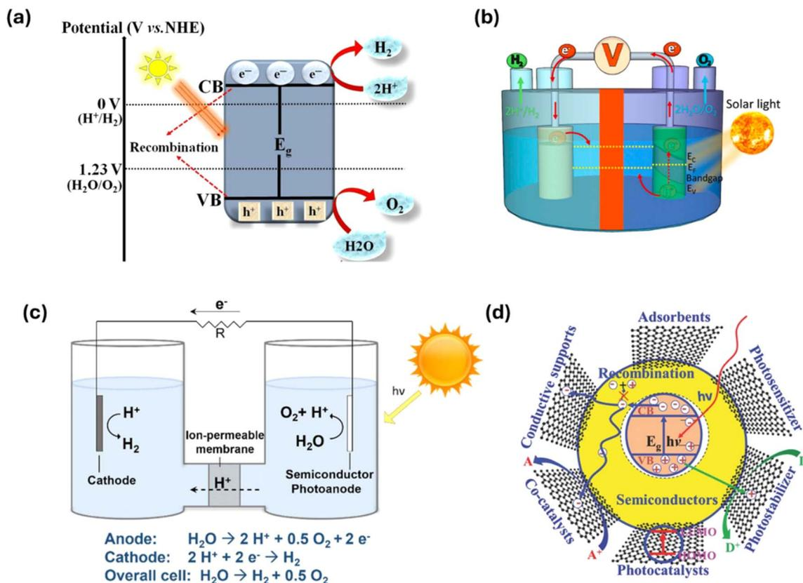
Fig. 11 (a) Illustrative overview of the general photocatalytic  $H_2$  generation mechanism. (b) Representation of photoanodes and cathode semiconductors for PEC  $H_2$  generation. (c) Mechanism of PEC water splitting for  $H_2$  generation. (d) Characteristics of graphene for photocatalytic and PEC  $H_2$  production.<sup>197–199</sup>
