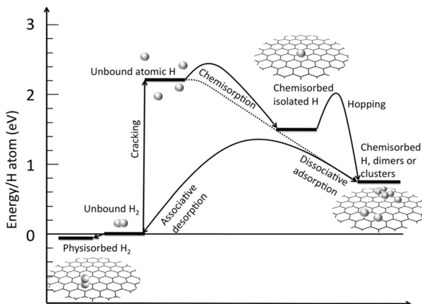
Fig. 13 Energy level diagram of hydrogen adsorption–desorption on the graphene monolayer.<sup>60</sup> Adapted with permission from RSC.
