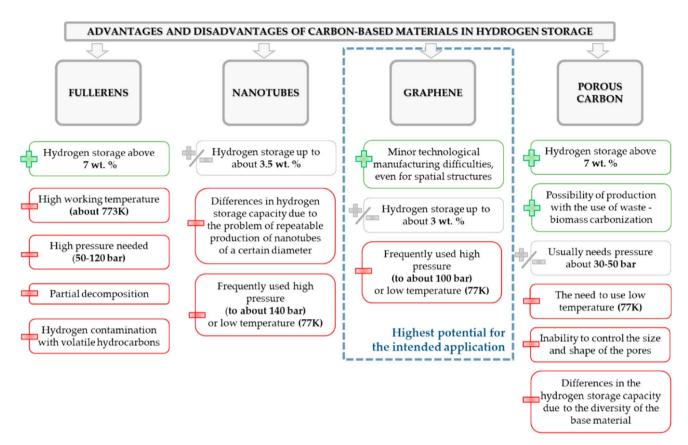
Fig. 14 Summary of solid-state hydrogen storage using different carbon-based materials.<sup>244</sup> Adapted with permission from MDPI.
