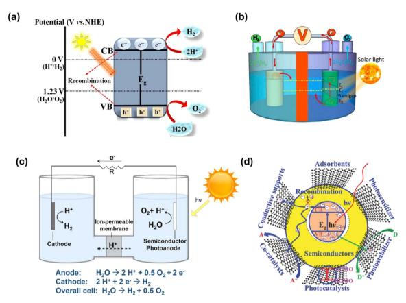
Fig. 11 (a) Illustrative overview of the general photocatalytic H<sub>2</sub> generation mechanism. (b) Representation of photoanodes and cathode semiconductors for PEC H<sub>2</sub> generation. (c) Mechanism of PEC water splitting for H<sub>2</sub> generation. (d) Characteristics of graphene for photocatalytic and PEC H<sub>2</sub> production. 197-199
