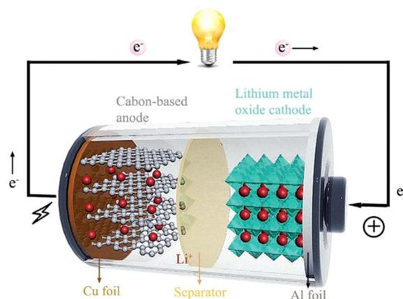
Fig. 1 Schematic of the structure and working mechanism of LIBs.<sup>66</sup>
