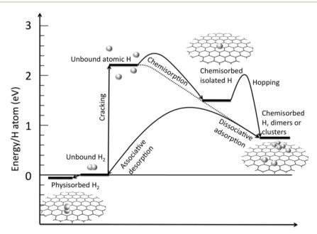
Fig. 13 Energy level diagram of hydrogen adsorption-desorption on the graphene monolayer.<sup>60</sup> Adapted with permission from RSC.
