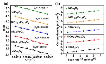
(a) Activation energy plots of OER and (b) scan-rate-dependent study of the synthesized materials
