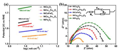
Fig. 7 (a) Tafel plots and (b) Nyquist plots with the equivalent circuit (shown in the inset) of the synthesized materials.
