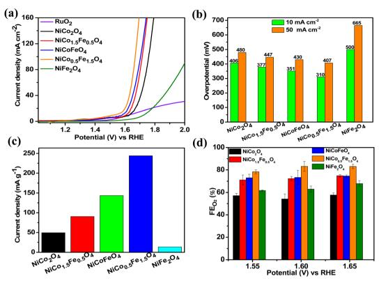
Fig. 5 (a) LSV polarisation plots; (b) overpotential at 10 and 50 mA cm<sup>-2</sup> current densities; (c) mass activities, and (d) FE(%) of oxygen evolution over the synthesized catalysts.
