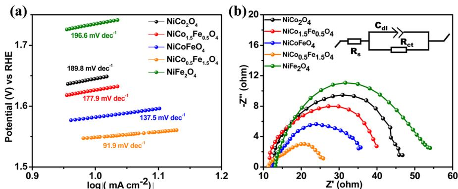
Fig. 7 (a) Tafel plots and (b) Nyquist plots with the equivalent circuit (shown in the inset) of the synthesized materials.
