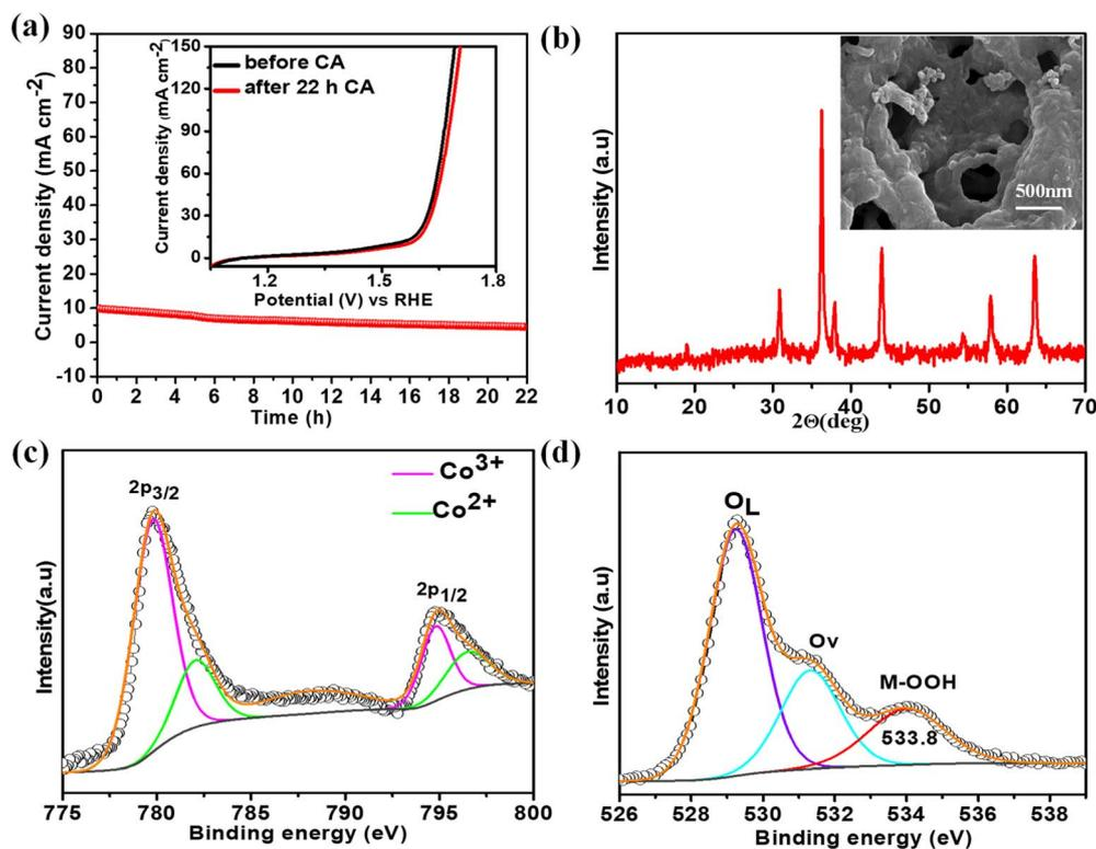
Fig. 8 (a) CA plots with polarisation curves of the fresh and exhausted  $\text{NiCo}_{0.5}\text{Fe}_{1.5}\text{O}_4$  in the inset; (b) XRD pattern with FE-SEM image of the exhausted  $\text{NiCo}_{0.5}\text{Fe}_{1.5}\text{O}_4$ ; (c) CO 2p and (d) O 1s spectra of the exhausted  $\text{NiCo}_{0.5}\text{Fe}_{1.5}\text{O}_4$ .
