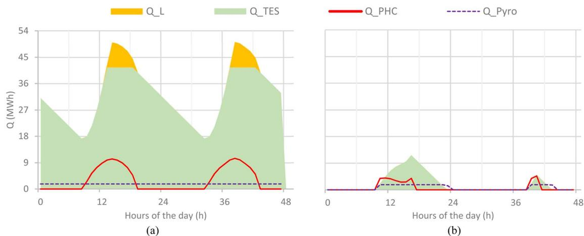
Fig. 8 Daily operation of the CSP-based pyrolysis plant with sand PHC,  $SM_T$  7 and 24 h TES size. Charts refer to (a) summer days (1–2 June) and (b) partially cloudy winter days (19–20 Jan).  $Q_{PHC}$ : energy transferred from CSP to PHC;  $Q_{TES}$ : stored energy;  $Q_L$ : lost solar energy;  $Q_{Pyro}$ : energy used in the pyrolyzer.
