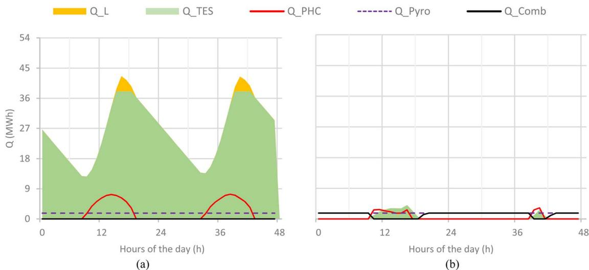
Fig. 9 Daily operation of the hybrid CSP pyrolysis plant with sand PHC, SMT 5 and 22 h TES size. Charts refer to (a) summer days (1–2 June) and (b) partially cloudy winter days (19–20 Jan). Q<sub>PHC</sub>: energy transferred from CSP to PHC; Q<sub>TES</sub>: stored energy; Q<sub>L</sub>: lost solar energy; Q<sub>Pyro</sub>: energy used in the pyrolyzer; Q<sub>Comb</sub>: energy generated by sludge and char combustion.
