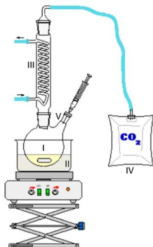
Fig. 2 Closed aging setup for accelerated laboratory aging (setup 2).
