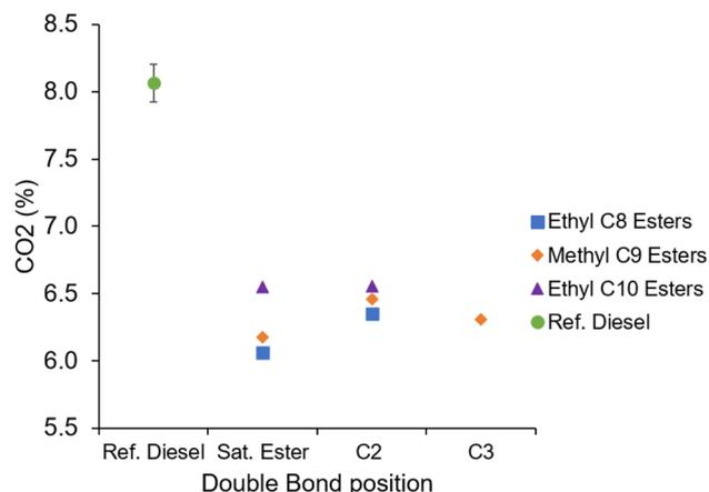
Fig. 16 Exhaust gas CO<sub>2</sub> emissions of the saturated and unsaturated esters, and reference diesel at constant injection timing and duration.
