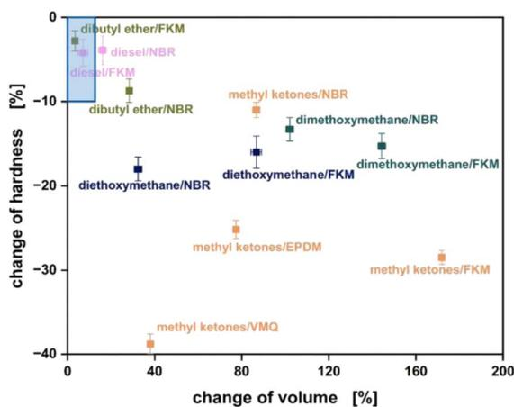
**Fig. 5** Change of volume and hardness for different bio-hybrid fuels and reference elastomer sealing materials. Light blue area shows the tolerance area for dynamic seals. FKM = fluorine kautschuk material; NBR = nitrile butadiene rubber; EPDM = ethylene propylene diene monomer rubber; VMQ = vinyl methyl silicone. The data are shown as mean values with standard deviations of six replicate measurements.
