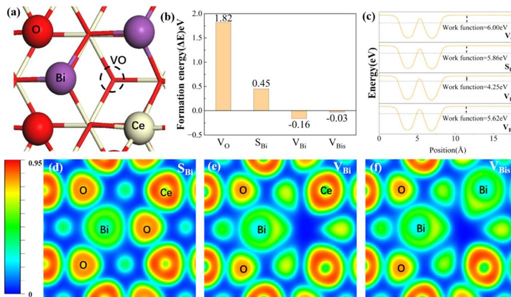
Fig. 1 (a) Configuration of four concept structures in  $\text{CeO}_2(111)$ . The formation energy (b), work function (c), and electron localization function (d–f) of the above four materials. White, red, and purple represent Ce, O, and Bi, respectively.
