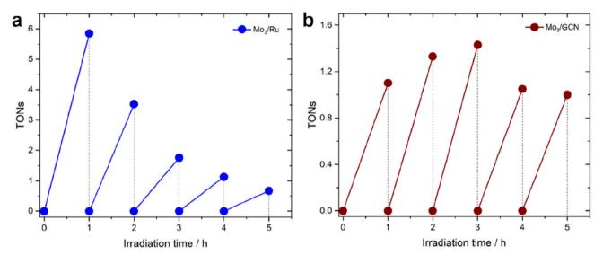
Fig. 5 Long-term HER profiles (in  $H_2A$ ) of (a)  $Mo_3/Ru$  system and (b)  $Mo_3/GCN$  system. TONs for the  $Mo_3/GCN$  system were calculated based on real loadings of  $[Mo_3S_{13}]^{2-}$  clusters on GCN mentioned in Table 1. The experiments were conducted using an LED 445 nm lamp (see Methods section 4.3 for more details).
