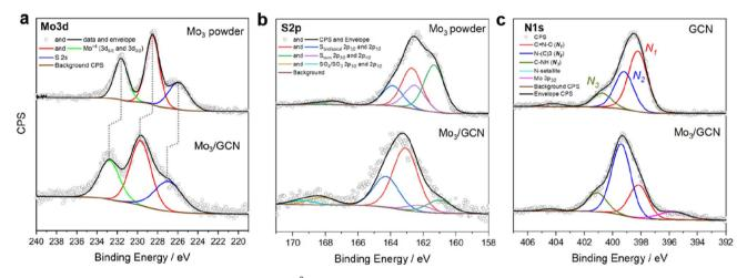
Fig. 3 XPS spectra of the Mo $_3$ /GCN cluster. The [Mo $_3$ S $_{13}$ ]<sup>2-</sup> clusters before (Mo $_3$  powder) and after (Mo $_3$ /GCN) attachment to the GCN surface, (a) Mo 3d, (b) S 2p, and (c) N 1s ( $N_1$ : pyridinic nitrogen;  $N_2$ : quaternary nitrogen;  $N_3$ : secondary amine), with corresponding fits.
