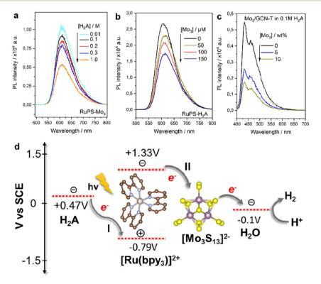
Fig. 4 PL emission spectra of the Mo<sub>3</sub>/Ru system with varying (a)  $H_2A$  and (b)  $[Mo_3S_{13}]^{2-}$  concentrations and (c)  $Mo_3/GCN$  system with varying  $[Mo_3S_{13}]^{2-}$  loadings and (d) schematic of reductive (I) and oxidative (II) quenching mechanisms of the  $[Ru(bpy)_3]^{2+}$  photosensitizer in the presence of the  $[Mo_3S_{13}]^{2-}$  catalyst and  $H_2A$  sacrificial donor. Energy levels are based on the relevant literature source.<sup>26</sup>
