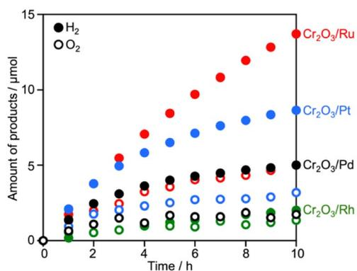
Fig. 2 Z-WS by the Cr<sub>2</sub>O<sub>3</sub>/M/CLTO-BiVO<sub>4</sub>-Co(bpy)<sub>3</sub>SO<sub>4</sub> system. Photocatalyst: 0.05 g each; reactant solution: 0.1 mM Co(bpy)<sub>3</sub>SO<sub>4</sub>, 160 mL; light source: 300 W Xe lamp ( $\lambda > 420$  nm).
