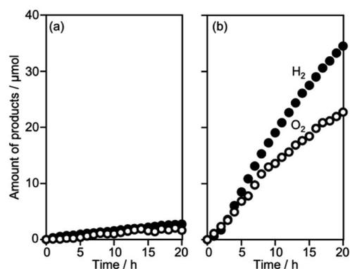
Fig. 8 Time courses of gas evolution by Z-scheme systems without the  $\text{Co}(\text{bpy})_3^{3+/2+}$  electron shuttle; (a)  $\text{Cr}_2\text{O}_3/\text{Ru}/\text{CLTO}-\text{BiVO}_4$  and (b)  $\text{Cr}_2\text{O}_3/\text{Ru}/\text{CLTO}-\text{RGO}/\text{BiVO}_4$ . Photocatalyst: 0.05 g each; reactant solution: water, 160 mL; light source: 300 W Xe lamp ( $\lambda > 420 \text{ nm}$ ).
