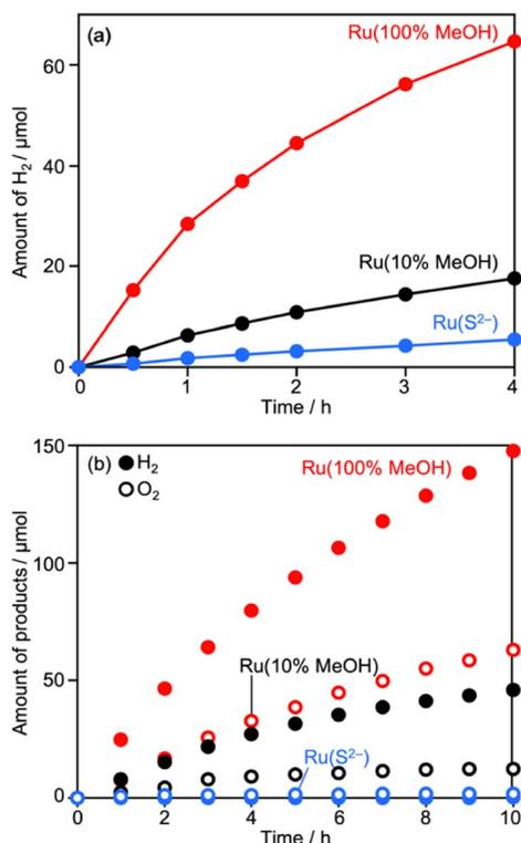
Fig. 3 Photocatalytic (a) H<sub>2</sub> evolution and (b) Z-WS using Cr<sub>2</sub>O<sub>3</sub> (1.2 wt%)/Ru (0.5 wt%)/CLTO prepared under different photodeposition conditions. Photocatalyst: 0.2 g for (a) and 0.05 g each for (b); reactant solution: 10 vol% methanol for (a) and 0.1 mM Co(bpy)<sub>3</sub>SO<sub>4</sub> for (b), 160 mL; light source: 300 W Xe lamp (λ >420 nm).
