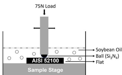
Fig. 2 Schematic diagram of the tribological experimental setup.
