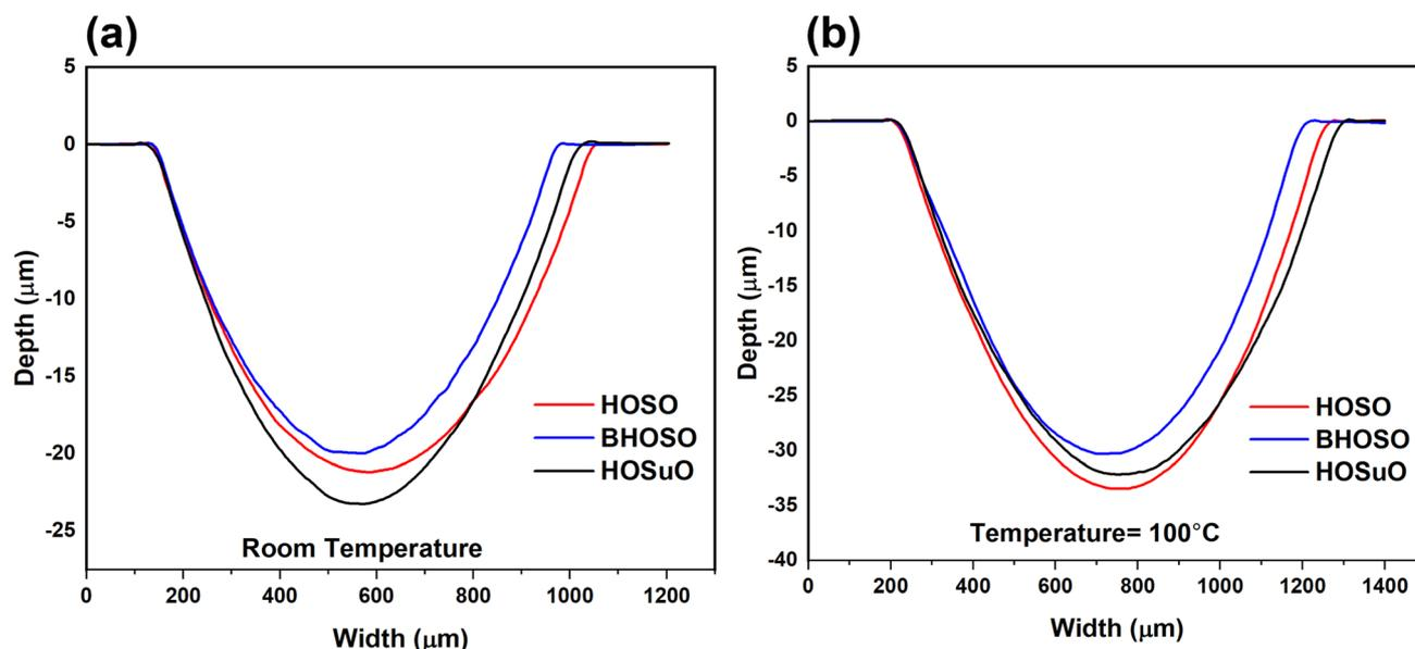
Fig. 9 Two-dimensional depth profiles of wear tracks captured along the transverse direction at (a) room temperature (b) 100 °C.
