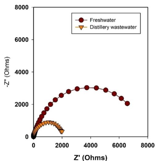
Fig. 5 Nyquist plots of  $\text{Ni}_2\text{Se}_3$  (anode) and Ni mesh (cathode) in both freshwater and distillery wastewater electrolytes. It is important to note that impedance measurements were conducted at open circuit potential.
