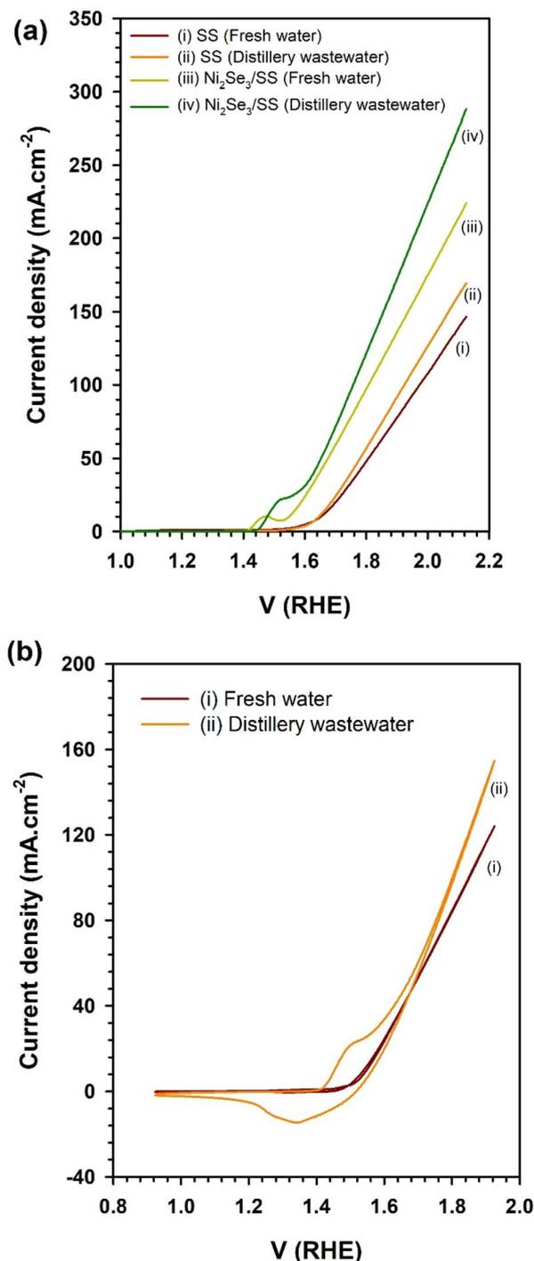
Fig. 3 (a) Linear sweep voltammogram results of stainless steel and  $\text{Ni}_2\text{Se}_3$  nanoparticles coated stainless steel substrates in freshwater and distillery wastewater electrolyte. (b) CV of  $\text{Ni}_2\text{Se}_3/\text{SS}$  anode in freshwater and distillery wastewater-based electrolyte. Note that the concentration of the electrolyte was  $1 \text{ M NaOH}$ .
