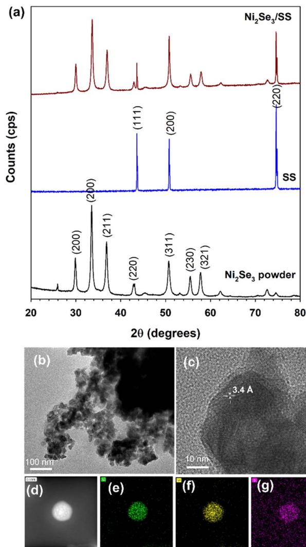
Fig. 1 (a) XRD pattern of  $\text{Ni}_2\text{Se}_3$  powder, stainless steel substrate (SS) and  $\text{Ni}_2\text{Se}_3$  coated SS ( $\text{Ni}_2\text{Se}_3/\text{SS}$ ). HRTEM images of  $\text{Ni}_2\text{Se}_3$  powder (b) at 100 nm scale and (c) 10 nm scale. (d) Elemental mapping of  $\text{Ni}_2\text{Se}_3$  uniformly dispersing the elements of (e) Ni, (f) Se and (g) O.
