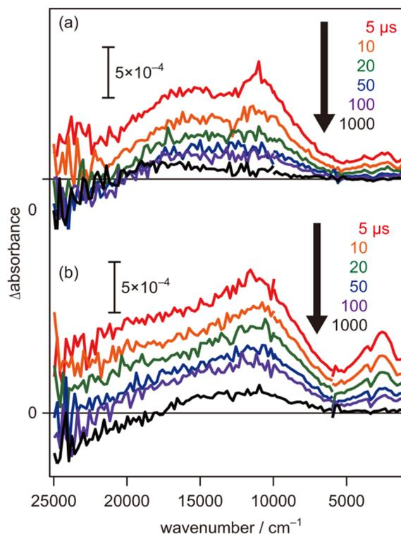
Fig. 4 Transient absorption spectra of (a) SrTiO<sub>3</sub>:Sc,Mg and (b) SrTiO<sub>3</sub>:Al powders irradiated by UV (355 nm) laser pulses in N<sub>2</sub> (2.7 kPa). The pump energy was 0.5 mJ per pulse, and the repetition rate was 5 Hz.
