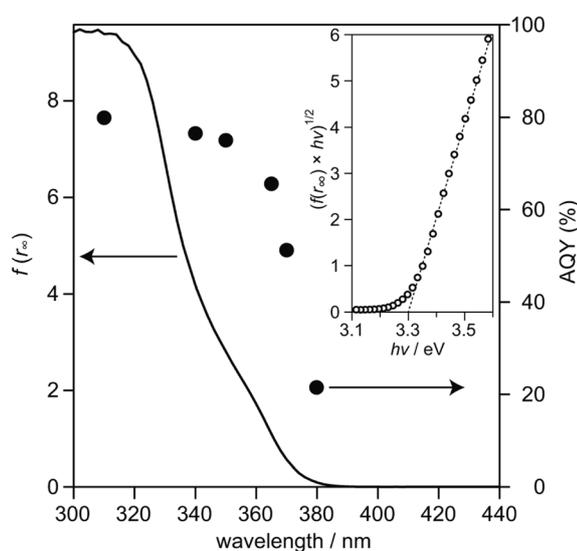
Fig. 3 DR spectra of SrTiO<sub>3</sub>:Sc,Mg (solid line) and AQYs during water splitting on SrTiO<sub>3</sub>:Sc,Mg loaded with Rh/Cr<sub>2</sub>O<sub>3</sub> HER and CoOOH OER cocatalysts (filled symbols). The inset shows a  $(f(r_\infty) \times hv)^{1/2}$  vs.  $hv$  plot obtained from the DR spectrum.
