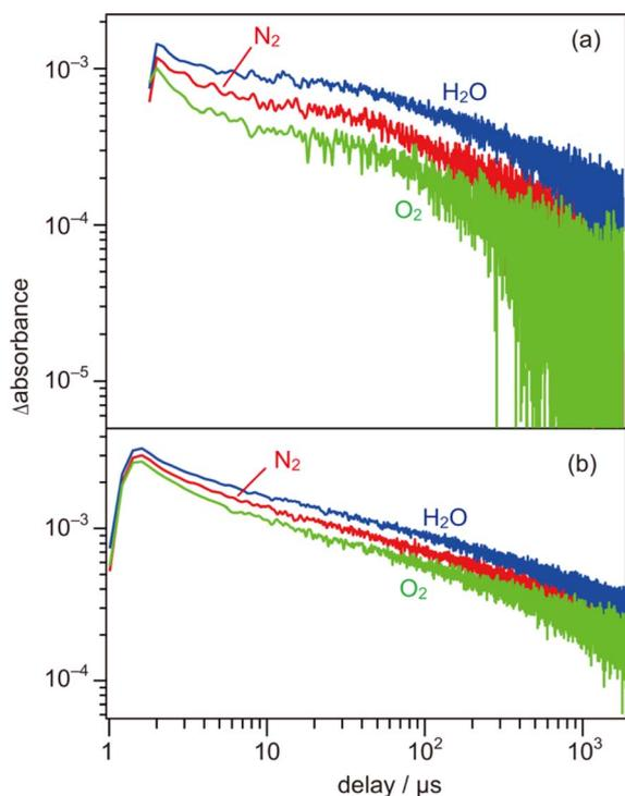
Fig. 5 Decay curves of the transient absorption of (a) SrTiO<sub>3</sub>:Sc,Mg and (b) SrTiO<sub>3</sub>:Al powders irradiated by 355 nm laser pulses (0.5 mJ per pulse at 0.2 Hz). The decay curves were  $11\,000\text{ cm}^{-1}$ , in N<sub>2</sub> (2.7 kPa), O<sub>2</sub> (2.7 kPa), and water vapor (2.7 kPa).
