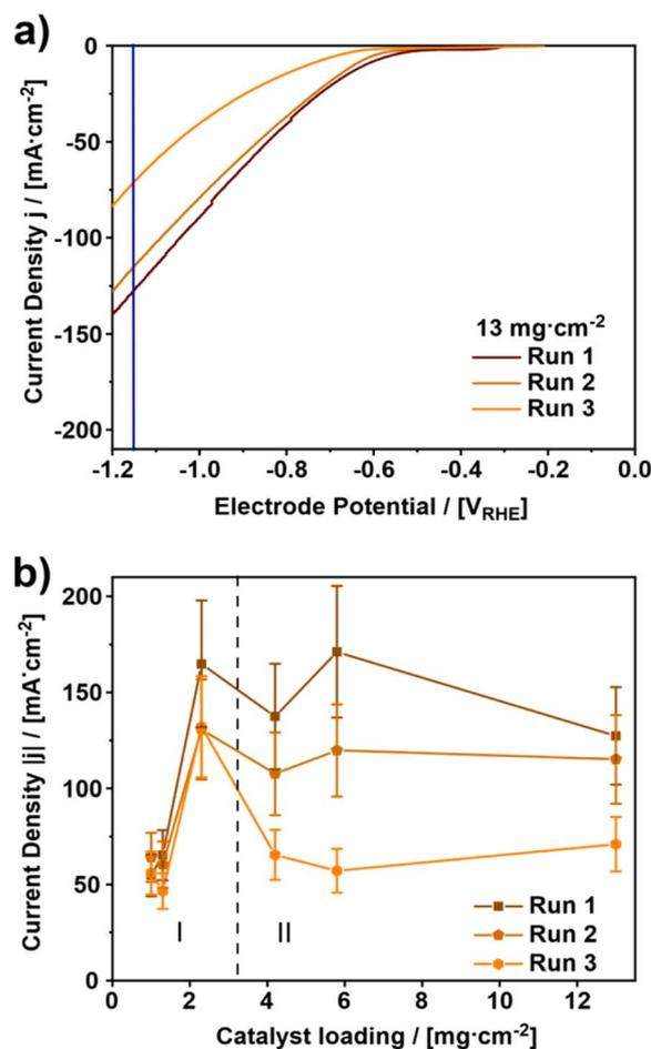
Fig. 2 (a) Exemplary course of the linear sweep voltammograms (LSVs) for the GDE with a catalyst loading of  $13 \text{ mg cm}^{-2}$ . (b) Evaluation of the cathodic current density at  $-1.15 V_{\text{RHE}}$  depending on the catalyst loading. (Measurement conditions: batch reactor, 12 ml electrolyte,  $1 \text{ M KHCO}_3$ , continuous  $\text{CO}_2$  supply of  $20 \text{ ml min}^{-1}$ , start at room temperature, electrolysis time: 45 min each).
