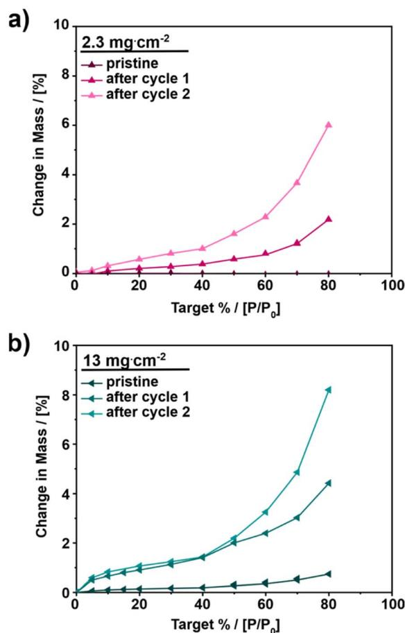
**Fig. 6** Vapor sorption measurements of GDEs with different catalyst loadings: (a) 2.3 mg cm<sup>-2</sup> and (b) 13 mg cm<sup>-2</sup>. Vapor adsorption isotherms of the investigated GDEs in different states – pristine, after cycle 1 and after cycle 2. Vapor sorption measurements were conducted at 25 °C with a relative humidity from 0 to 80%; each humidity point was held for 60 min.
