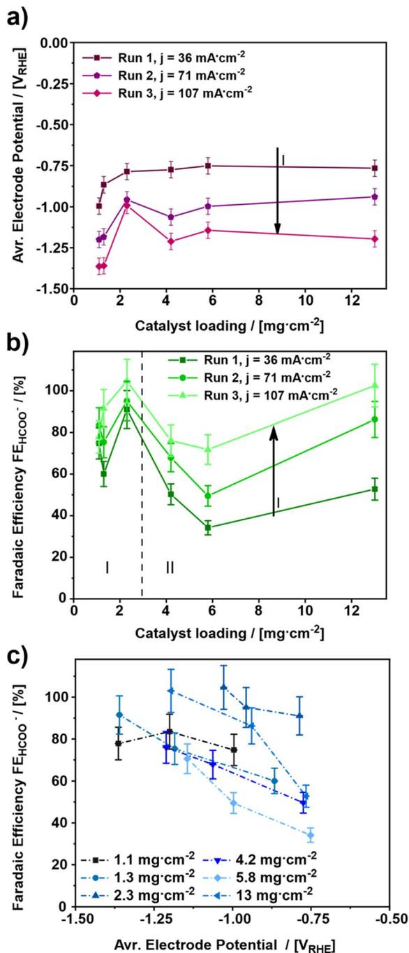
Fig. 1 Influence of the catalyst loading on (a) the average electrode potential for three different applied current densities (36, 71 and 107 mA cm<sup>-2</sup>) and (b) the faradaic efficiency for formate after a run time of 11 min each. (c) Shows a combination of the plots a and b. (Measurement conditions: batch reactor, 12 ml electrolyte, 1 M KHCO<sub>3</sub>, continuous CO<sub>2</sub> supply of 20 ml min<sup>-1</sup>, start at room temperature, electrolysis time: 45 min each).
