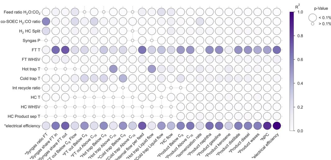
Fig. 3 Correlation matrix showing the coefficient of determination ( $R^2$ ) and the statistical significance based on the  $p$ -value for 43 959 samples. Due to the large sample size, a  $p$ -value of  $<0.001$  (0.1%) is chosen as the criterion for statistical significance.
