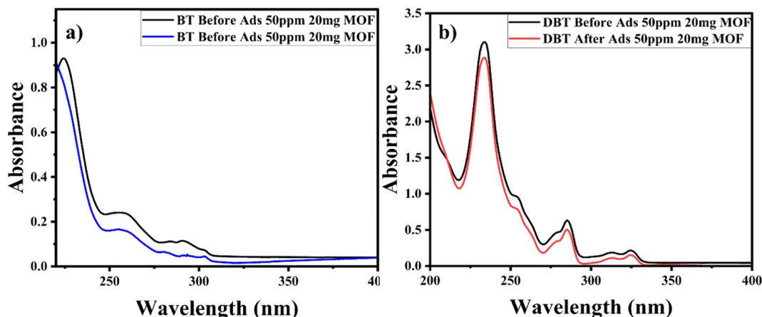
Fig. 10 UV-Vis spectra before and after adsorption of other sulfur-containing aromatic compounds with 20 mg adsorbent dosage and 50 mg L<sup>-1</sup> concentration of (a) benzothiophene (BT) and (b) dibenzothiophene (DBT).
