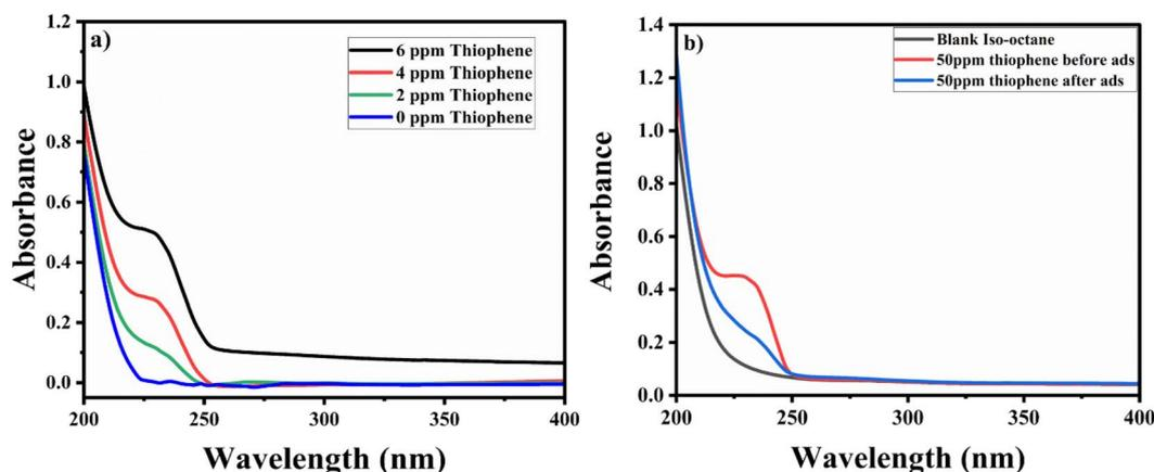
Fig. 2 (a) UV-Vis absorption spectra of different concentrations of thiophene with  $\lambda_{\text{max}}$  at 233 nm (0 to 6  $\text{mg L}^{-1}$ ). (b) UV-Vis absorption spectra of thiophene before and after adsorption.
