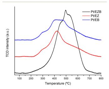
Fig. 3 Temperature programmed reduction of Pt/E catalysts.
