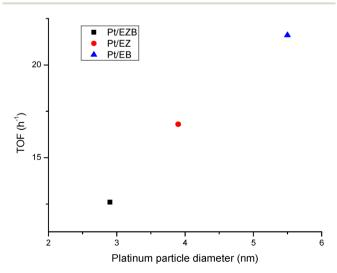
Fig. 6 Dependence of TOF on platinum particle size.
