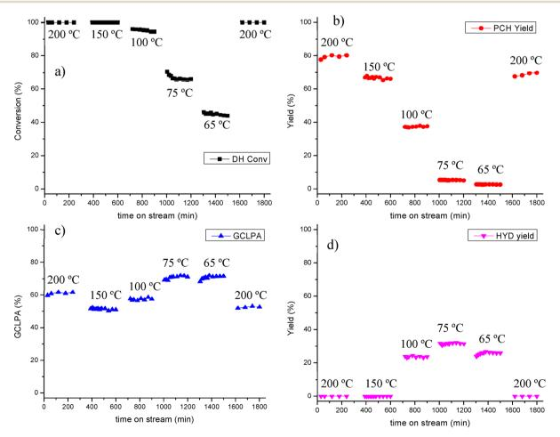
Fig. 7 Transformations of isoeugenol using Pt/EZB in a continuous reactor at different temperatures, 30 bar of H<sub>2</sub> liquid flow of 0.5 mL min<sup>-1</sup> and gas flow of 40 mL  $min^{-1}$  (a) dihydroeugenol conversion, (b) propylcyclohexane yield, (c) GCLPA and (d) hydrogenated intermediate yield as a function of time on stream.
