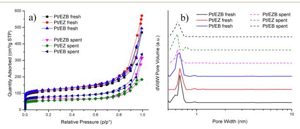
Fig. 2 (a) Adsorption-desorption isotherms and (b) pore size distribution of the fresh and spent Pt/E catalysts.
