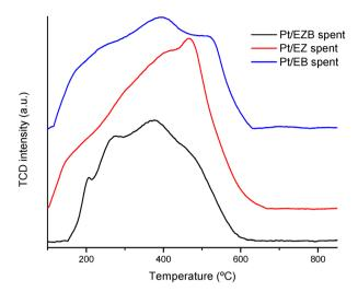
Temperature programmed oxidation of Pt/E catalysts.
