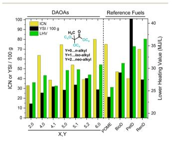
Fig. 1 Graphical comparison of  $C_2$ - $C_6$  DAOA and reference fuel combustion properties. ICN for DAOA-1 (X = 2, Y = 0) is <33 and shown for illustrative purposes. POME = "BB, n = 1-6", BioD = FAME biodiesel, PetD = petroleum diesel; RenD = renewable diesel from hydroprocessed esters and fatty acids (HEFA) process
