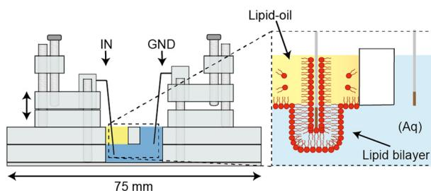
**A handheld laser-cut device for the size-controlled assembly and electrical characterisation of lipid bilayers**
