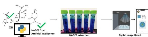
**Detection of surfactants using a hydrophobic natural deep eutectic solvent and smartphone**
