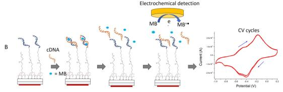
Fig. 1 DNA biosensor: A) representative thermographs of the photothermal module during different phases: laser-OFF, hybridization and MB release phase (laser ON, power 1.8 W) and dsDNA denaturation phase (laser ON, power 5 W). B) ITO-Sil-DNA module: surface-hybridization/MB interaction, dsDNA/MB denaturation and MB electrochemical detection.
