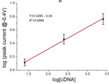
Fig. 6 DNA biosensor sensitivity test: A) CV cycles of DNA biosensor for the detection of different amounts of cDNA (0, 25, 250 and 2500 nM) in KCl 0.1 M (scan rate 0.01 V s<sup>-1</sup>; 25 °C); B) log-log linear response of the peak current ( $\mu$ A) at -0.4 V *versus* cDNA (nM), (Y = 0.328X - 0.34;  $R^2 = 0.9969$ ).
