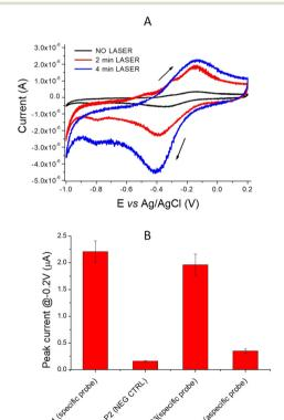
Fig. 5 DNA biosensor CV experiments: A) CV cycles for the detection of cDNA 250 nM in KCl 0.1 M (scan rate 0.01 V s $^{-1}$ ; 25 °C) at different photothermal conditions: no laser, laser 5 W for 2 min and laser 5 W for 4 min; B) specificity tests, peaks current at -0.4 V for each investigated spots: P1 (specific probe), P2 (negative control), P3 (specific probe) and P4 (aspecific probe).
