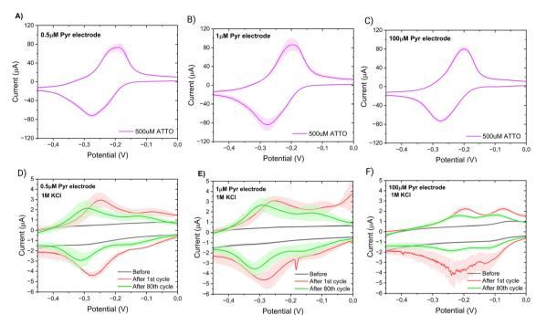
Fig. 7 Passivation against methylene blue of a SWCNTs electrode with different linker concentrations. CV response of passivated electrodes to 500  $\mu$ M of methylene blue (ATTO) (A-C) (N = 3). CV response of passivated electrodes in background (KCl) before and after the exposure of the electrodes to methylene blue (D-F) (N = 3).
