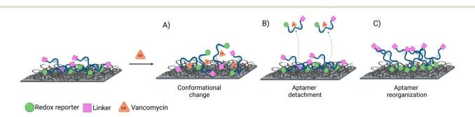
Fig. 5 Scheme of the three possible scenarios producing a signal change upon target addition: A) conformational change of the aptamer, B) detachment of the non-covalently bound aptamers, and/or C) reorganization of the non-covalently attached aptamers.
