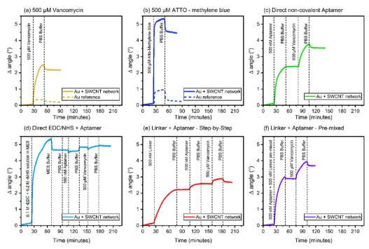
Fig. 3 SPR sensograms showing the adsorption of (a) 500  $\mu$ M vancomycin, (b) 500  $\mu$ M ATTO-MB2, (c) 500 nM aptamer *via* direct non-covalent binding, (d) direct covalent activation followed by 500 nM aptamer, (e) 500 nM linker followed by 500 nM aptamer (LbL approach) and (f) 500 nM linker + 500 nM aptamer – pre-mixed solution. The responses of adsorbed aptamers to buffer rinse and 500  $\mu$ M vancomycin injection were also followed for each aptamer linking protocol (c-f).
