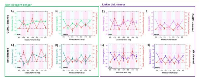
Fig. 6 Stability upon repetitive measurements of vancomycin at 40 and 2000 Hz of non-covalent sensors previously cleaned with GuHCl (A and B) and without a previous cleaning (C and D). Additionally, the stability upon repetitive measurements of vancomycin at 40 and 2000 Hz of linker LbL sensors previously cleaned with GuHCl (E and F) and with VA cleaning (G and H) is presented. The stability was assessed in terms of signal and peak position changes (N = 3).
