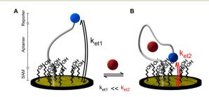
Fig. 1 Working principle of an ideal electrochemical aptamer-based sensor in A) the absence and B) presence of target.<sup>5</sup>
