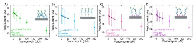
Fig. 8 Calibration curves and linear fit from 1–50 μM VA for A) direct noncovalent, B) direct covalent, C) linker LbL, and D) linker premix electrodes ( $l_{pa}$  = forward partial peak current, c = vancomycin concentration, LOD = limit of detection, N = 3).
