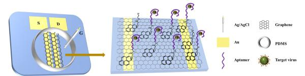
Fig. 1 Schematic diagram of Aptamer-GFET sensor.
