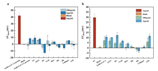
Fig. 4 (a)  $\Delta V_{\text{Dirac}}$  response of SARS-CoV-2 GFET biosensor to SARS-CoV-2 spike protein in the presence of other interfering substances. (b)  $\Delta V_{\text{Dirac}}$ response of norovirus GFET biosensor to norovirus-like particles in the presence of other interfering substances. Error bars represent the standard deviation calculated from a minimum of three independent measurements (n = 3).
