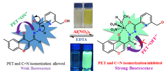
Fig. 6 Probable sensing mechanism of HMCP with \text{Al}^{3+} .
