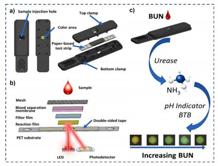
Fig. 8 (a) Schematic diagram of a disposable photochemical test strip; (b) the composition of the multilayer film strip and a schematic diagram of reflectance photometry; (c) the principle of the enzymatic colorimetric reaction.<sup>65</sup> Copyright 2023, Elsevier.
