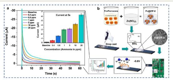
Fig. 3 Schematic illustration of amperometric electrochemical biosensors for ammonia detection. (a) Diffusion-limited chronoamperometry. Calibrated dose-response chronoamperograms for ammonia gas concentration ranging from 400 ppb to 20 ppm. (b) Schematic representation of the optimized preparation approach of Fc@ZIF-8-modified SENCE.<sup>37</sup> Copyright 2021, American Chemical Society.
