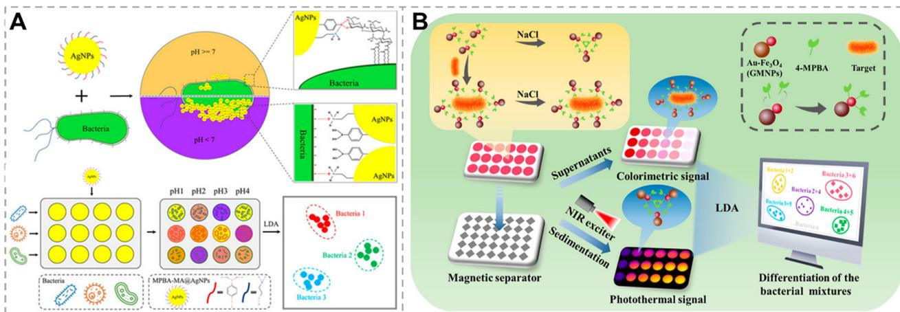
**Fig. 4** Bacterial recognition through the interaction between boronic acid and the *cis*-diol group. A) A colorimetric sensor array based on Wulff-type boronate functionalized AgNPs for bacterial identification. Reproduced with permission.<sup>60</sup> Copyright 2019, American Chemical Society. B) A dual-mode sensor array based on colorimetric and photothermal detection for bacterial identification. Reproduced with permission.<sup>62</sup> Copyright 2023, American Chemical Society.
