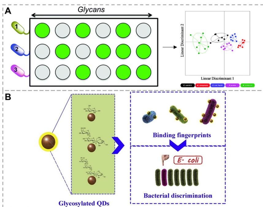
**Fig. 5** Bacterial recognition through the interaction between lectins and glycan. A) Discrimination of bacteria by ratiometric analysis of their carbohydrate binding profile. Reproduced with permission.<sup>68</sup> Copyright 2016, Royal Society of Chemistry. B) A sensor array consisting of multivalent glycosylated Cu:CdS quantum dots for rapid bacterial discrimination. Reproduced with permission.<sup>69</sup> Copyright 2017, Elsevier.
