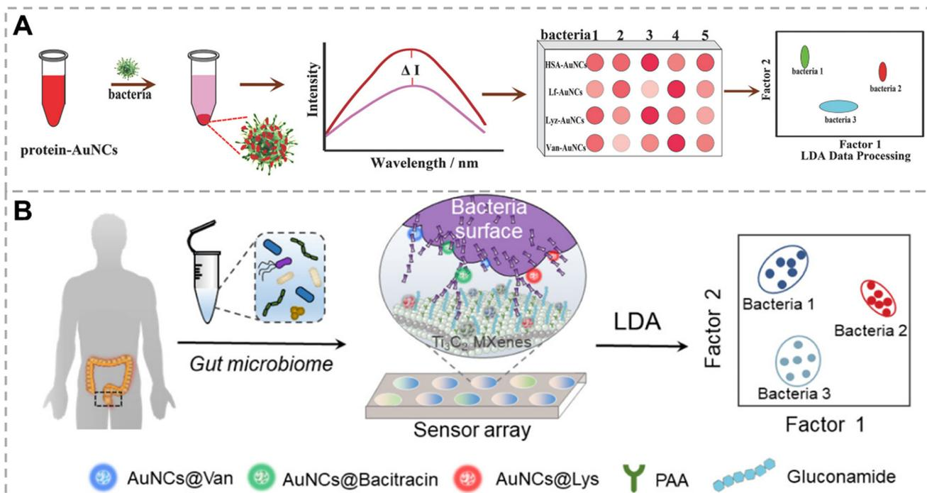
**Fig. 7** Bacterial recognition through the interaction between proteins and specific receptors on bacterial surfaces. A) Protein-AuNC-based fluorescence sensor array for discrimination of bacteria. Reproduced with permission.<sup>78</sup> Copyright 2018, Wiley-VCH. B) Multichannel sensor array based on multi-functionalized AuNCs for gut microbiota detection. Reproduced with permission.<sup>83</sup> Copyright 2023, American Chemical Society.
