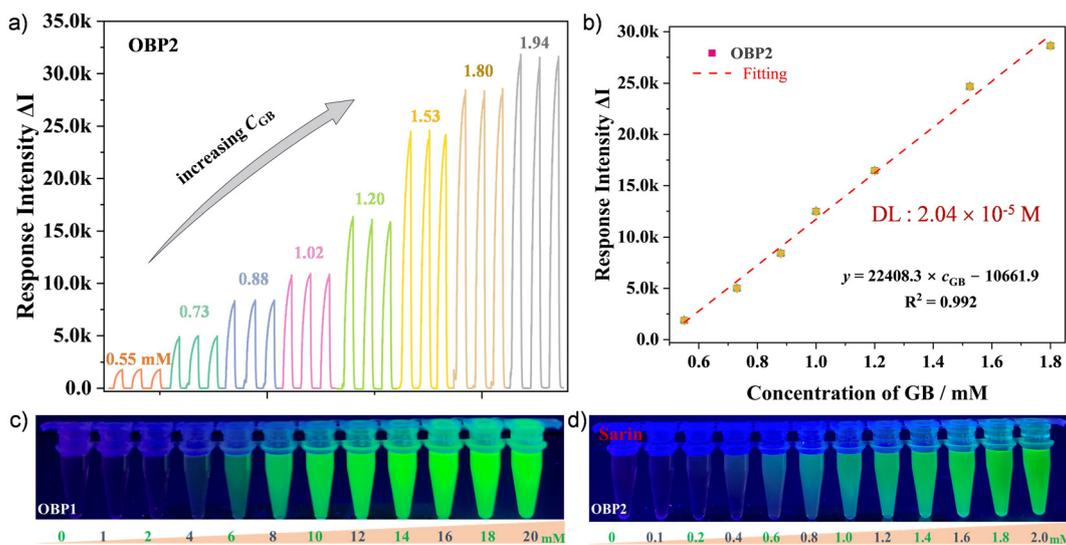
**Fig. 6** (a) Response traces of OBP2 in ACN to different concentrations of GB conducted by the home-made compact device prototype. (b) Response plot and linear fitting of OBP2 to different concentrations of GB. Fluorescence color changes of compound OBP1 (c) and OBP2 (d) to sarin (GB).
