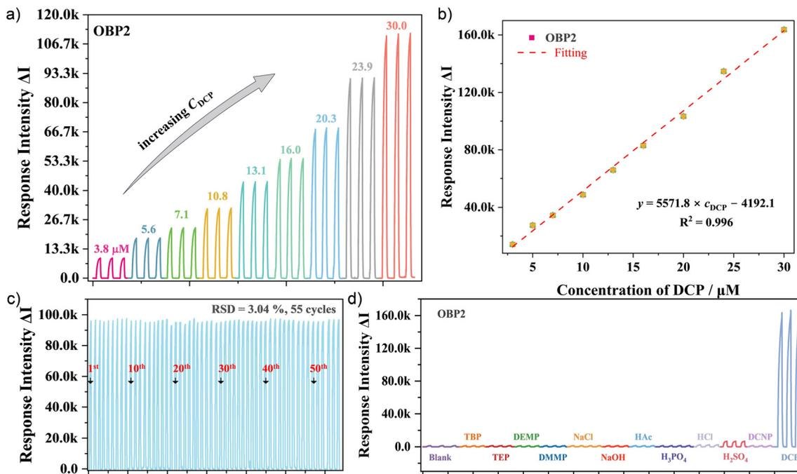
**Fig. 5** (a) Response traces of OBP2 in ACN to different concentrations of DCP conducted by the compact device (note: each test was repeated at least three times). (b) Response plot and linear fitting of OBP2 to different concentrations of DCP. (c) Sensing reversibility and stability tests of the sensing platform toward DCP with 55 cycles. (d) Response selectivity of OBP2 to the presence of different potential interferents ( $c \sim 30.0 \mu\text{M}$ ).
