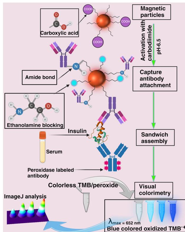
**Scheme 1** Conceptual schematic illustration of the colorimetric immunosensor developed in this report for insulin detection in biofluids.
