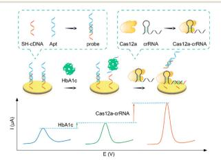
1 Schematic illustration CRISPR-amplified а electrochemical aptasensor for HbA1c detection.
