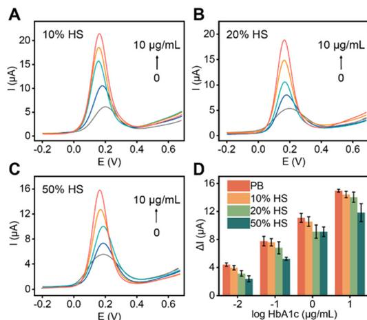
**Fig. 5** SWV curves of this CRISPR-amplified aptasensor for the detection of different concentrations of HbA1c in (A) 10% human serum, (B) 20% human serum and (C) 50% human serum. (D)  $\Delta I$  of the aptasensor was tested in PB, 10%, 20% and 50% human serum for the detection of 0.01, 0.1, 1 and 10  $\mu\text{g mL}^{-1}$  HbA1c.
