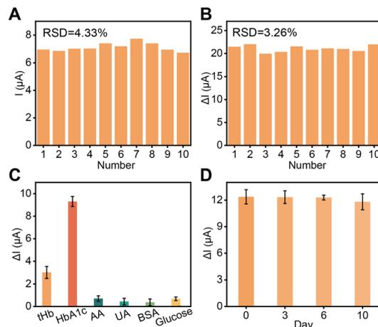
**Fig. 4** (A) SWV responses of ten independent CRISPR-amplified aptasensors for HbA1c detection under the same conditions. (B)  $\Delta I$  of ten independent CRISPR-amplified aptasensors for 100 µg mL<sup>-1</sup> HbA1c detection. (C)  $\Delta I$  of this aptasensor for the detection of tHb, HbA1c, AA, UA, BSA and glucose. (D) The storage stability of this aptasensor. The error bars represent the standard deviation of at least three independent measurements.
