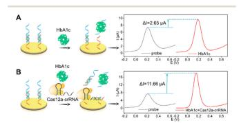
**Fig. 2** Schematics and electrochemical signal change of the (A) CRISPR-free aptasensor and (B) CRISPR-amplified aptasensor for HbA1c detection in 0.5 mM [Fe(CN)<sub>6</sub>]<sup>3-/4-</sup> solution containing 0.1 M KCI
