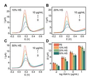
Fig. 5 SWV curves of this CRISPR-amplified aptasensor for the detection of different concentrations of HbA1c in (A) 10% human serum. (B) 20% human serum and (C) 50% human serum. (D)  $\Delta I$  of the aptasensor was tested in PB, 10%, 20% and 50% human serum for the detection of 0.01, 0.1, 1 and 10 µg mL<sup>-1</sup> HbA1c.
