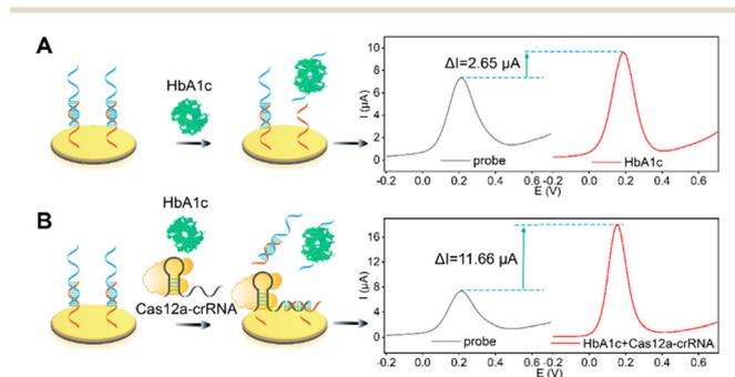
Fig. 2 Schematics and electrochemical signal change of the (A) CRISPR-free aptasensor and (B) CRISPR-amplified aptasensor for HbA1c detection in 0.5 mM  $[\text{Fe}(\text{CN})_6]^{3-/4-}$  solution containing 0.1 M KCl.
