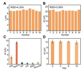
Fig. 4 (A) SWV responses of ten independent CRISPR-amplified aptasensors for HbA1c detection under the same conditions. (B)  $\Delta I$  of ten independent CRISPR-amplified aptasensors for 100  $\mu g$  mL $^{-1}$  HbA1c detection. (C)  $\Delta I$  of this aptasensor for the detection of tHb, HbA1c, AA, UA, BSA and glucose. (D) The storage stability of this aptasensor. The error bars represent the standard deviation of at least three independent measurements.
