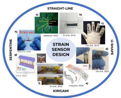
Fig. 5 Strain sensor design and shape. (a and b) Straight line strain sensor, <sup>37,71</sup> (c and d) U-shape strain sensor, <sup>72,74</sup> (e and f) kirigami strain sensor, <sup>47,75</sup> (g and h) serpentine strain sensor.
