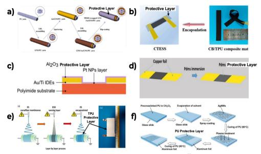
Fig. 4 Examples of protective encapsulation layers. (a) PDMS-wrapped GNS/Au/GNS/PU yarn, 65 (b) CB/TPU/Ecoflex strain sensor (CTESS), 67 (c) alumina as protective layer, 68 (d) PDMS-encapsulated MXene@polyester fabric strain sensor, 66 (e) stretchable MXene/thermoplastic polyurethanebased strain sensor, <sup>69</sup> (f) PU as protective layer of the sandwich structured PU/AgNW/PU composite strain sensor. <sup>70</sup>
