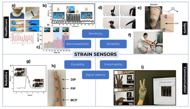
Fig. 1 (a) Measurements of human body induced deformations, 1 (b) finger gesture detection, 2 (c) measurements of different angles of bending finger,<sup>3</sup> (d) classification of training exercise,<sup>4</sup> (e) joint angle detection,<sup>5</sup> (f) sweat monitoring,<sup>6</sup> (g) strain sensing for robot hand,<sup>8</sup> (h) strain sensors on prosthetic finger, 9 (i) sign language translation. 11
