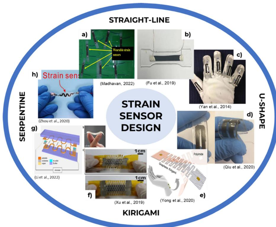
Fig. 5 Strain sensor design and shape. (a and b) Straight line strain sensor,<sup>37,71</sup> (c and d) U-shape strain sensor,<sup>72,74</sup> (e and f) kirigami strain sensor,<sup>47,75</sup> (g and h) serpentine strain sensor.<sup>73,76</sup>
