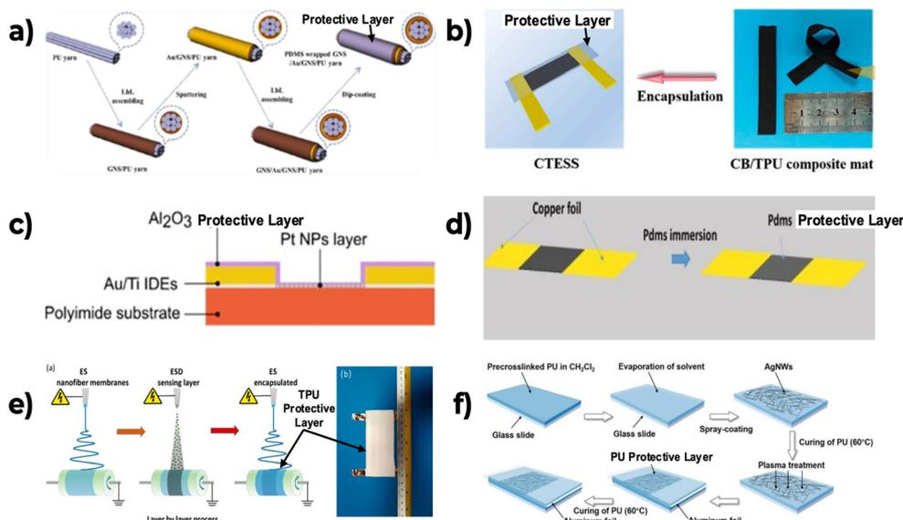
Fig. 4 Examples of protective encapsulation layers. (a) PDMS-wrapped GNS/Au/GNS/PU yarn,<sup>65</sup> (b) CB/TPU/Ecoflex strain sensor (CTESS),<sup>67</sup> (c) alumina as protective layer,<sup>68</sup> (d) PDMS-encapsulated MXene@polyester fabric strain sensor,<sup>66</sup> (e) stretchable MXene/thermoplastic polyurethane-based strain sensor,<sup>69</sup> (f) PU as protective layer of the sandwich structured PU/AgNW/PU composite strain sensor.<sup>70</sup>
