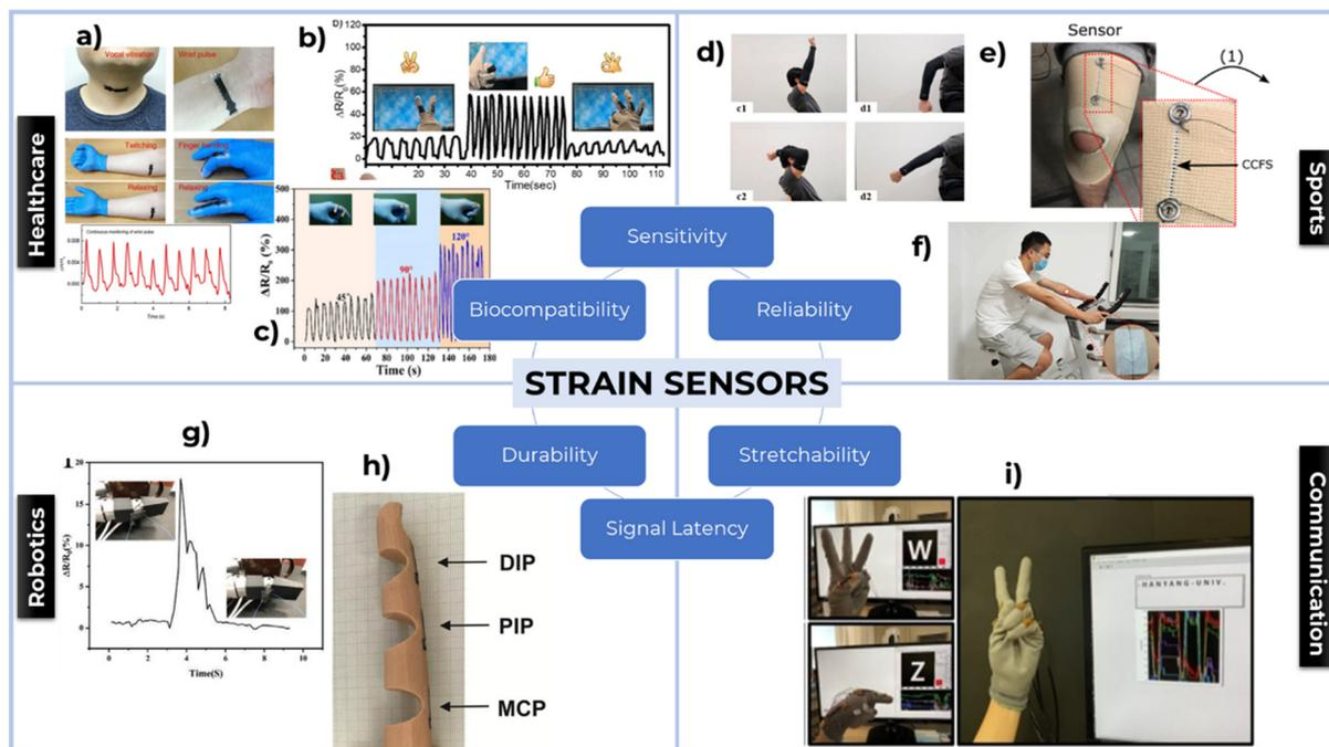
**Fig. 1** (a) Measurements of human body induced deformations,<sup>1</sup> (b) finger gesture detection,<sup>2</sup> (c) measurements of different angles of bending finger,<sup>3</sup> (d) classification of training exercise,<sup>4</sup> (e) joint angle detection,<sup>5</sup> (f) sweat monitoring,<sup>6</sup> (g) strain sensing for robot hand,<sup>8</sup> (h) strain sensors on prosthetic finger,<sup>9</sup> (i) sign language translation.<sup>11</sup>
