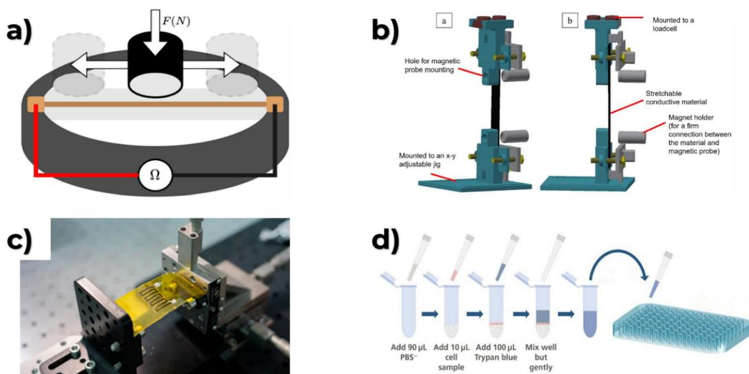
**Fig. 7** Equipment for evaluating strain sensor performance. (a) Abrasion tester,<sup>82</sup> (b) tensile machine,<sup>83</sup> (c) electro-mechanical tester for bending test,<sup>84</sup> (d) trypan blue assay.<sup>85</sup>
