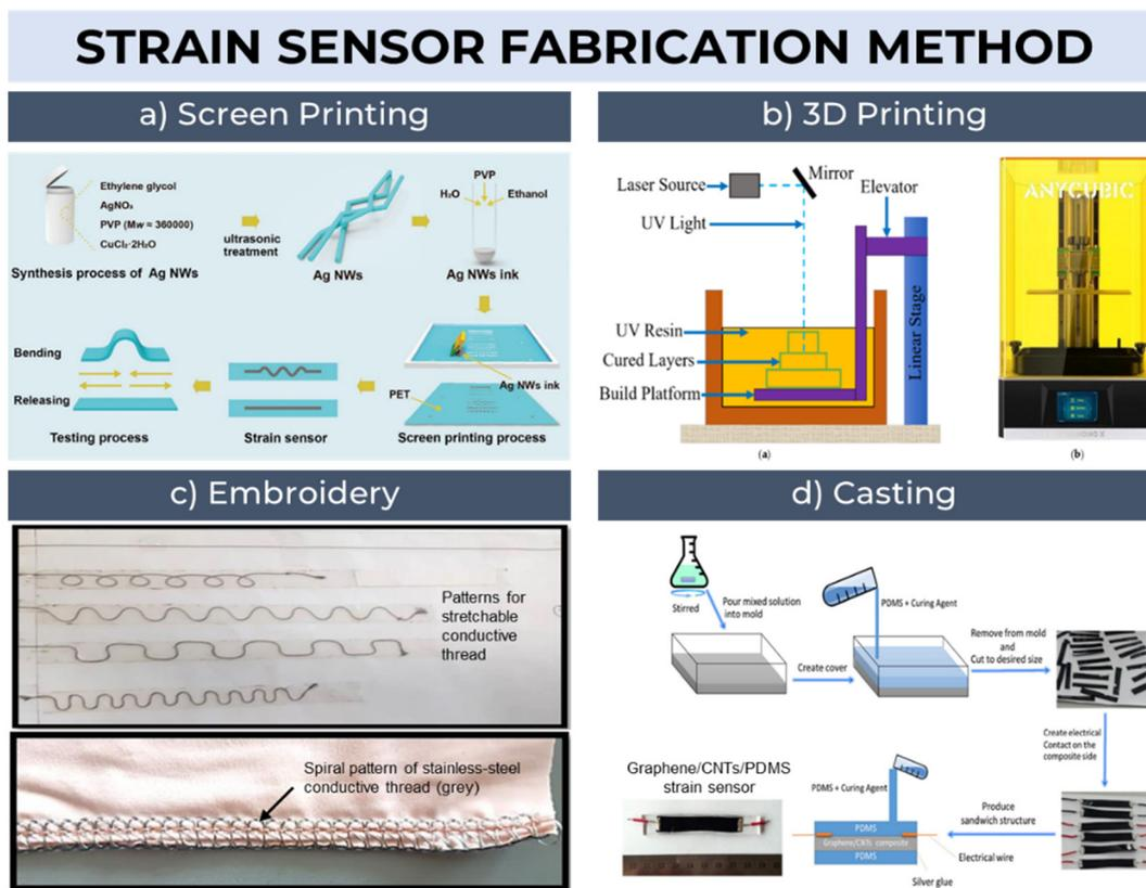
Fig. 3 Fabrication method of strain sensor. (a) Strain sensor screen printing process flow.<sup>50</sup> (b) 3D printing using UV resin material.<sup>51</sup> (c) Embroidery patterns sewn on fabric using conductive thread.<sup>52</sup> (d) Casting process flow of strain sensor.<sup>53</sup>
