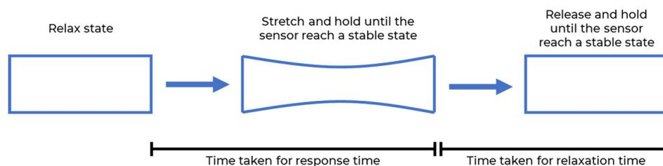
Fig. 8 Signal latency test.
