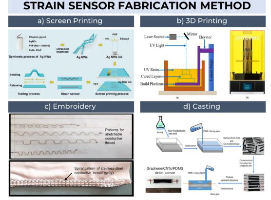
Fig. 3 Fabrication method of strain sensor. (a) Strain sensor screen printing process flow.<sup>50</sup> (b) 3D printing using UV resin material.<sup>51</sup> (c) Embroidery patterns sewn on fabric using conductive thread.<sup>52</sup> (d) Casting process flow of strain sensor.<sup>53</sup>
