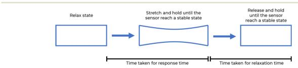
Fig. 8 Signal latency test.
