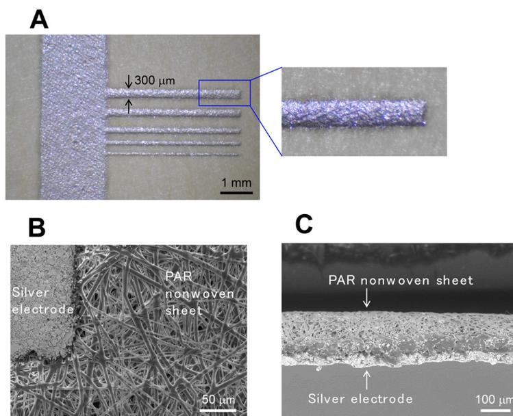
Fig. 5 Stereomicroscopic and SEM images of the fabricated  $\mu\text{PADs-NW}$ . (A) Stereomicroscopic images of comb electrodes screen-printed with different widths and its magnified view. (B) SEM image of the PAR nonwoven sheet surface in the vicinity of the silver electrode. (C) Cross-sectional SEM image of the electrode area.
