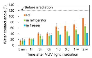
Fig. 6 Change of the water contact angle over time following VUV light irradiation.
