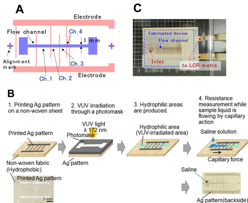
**Fig. 1** Device design and fabrication processes. (A) Design drawing, (B) fabrication processes (upper) and device photos (lower) of  $\mu\text{PAD-NWs}$ , and (C) photograph of the measurement setup.
