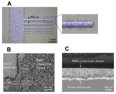
Fig. 5 Stereomicroscopic and SEM images of the fabricated  $\mu$ PADs-NW. (A) Stereomicroscopic images of comb electrodes screen-printed with different widths and its magnified view. (B) SEM image of the PAR nonwoven sheet surface in the vicinity of the silver electrode. (C) Cross-sectional SEM image of the electrode area.
