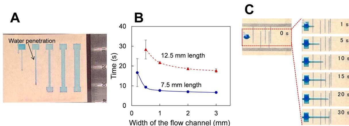
**Fig. 3** Examples of differences in the flow time based on the channel width, and time lapse of liquid flow. (A) View of channels with the channel widths of 0.5, 1, 2, and 3 mm. (B) Dependence of the elapsed time on the channel width to the lengths of 7.5 mm (blue) and 12.5 mm (red). (C) Time lapse photographs of colored water flow in a channel with electrodes.
