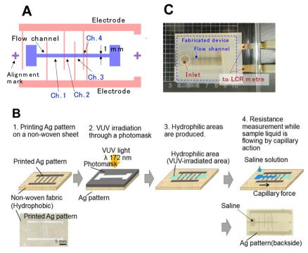
Fig. 1 Device design and fabrication processes. (A) Design drawing, (B) fabrication processes (upper) and device photos (lower) of μPAD-NWs, and (C) photograph of the measurement setup.
