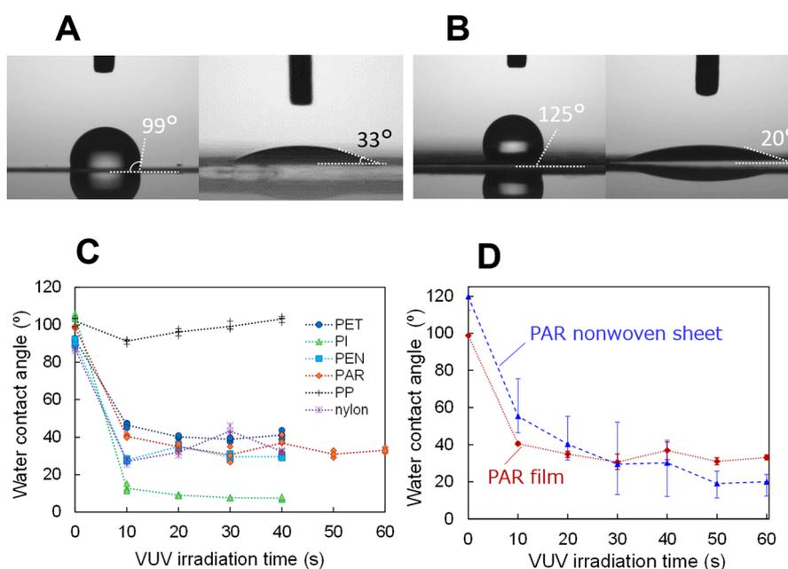
**Fig. 2** Differences in the water contact angle before and after VUV irradiation on polymer films and a PAR nonwoven sheet. (A) Water contact angles before (left) and after (right) 60 s of VUV light irradiation on a PAR film and (B) PAR nonwoven sheet. (C) Water contact angles for various polymer films at different VUV light exposure times, and for a (D) PAR film and a nonwoven sheet.
